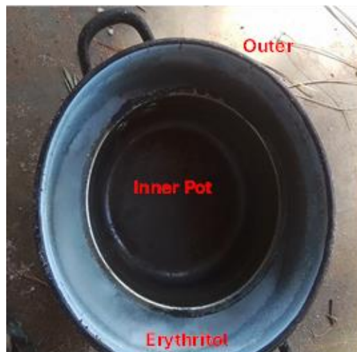
Figure 2. A Photograph showing the open inner and outer pots using 2 kg erythritol as the storage material. The same configuration was used with iron filings.
