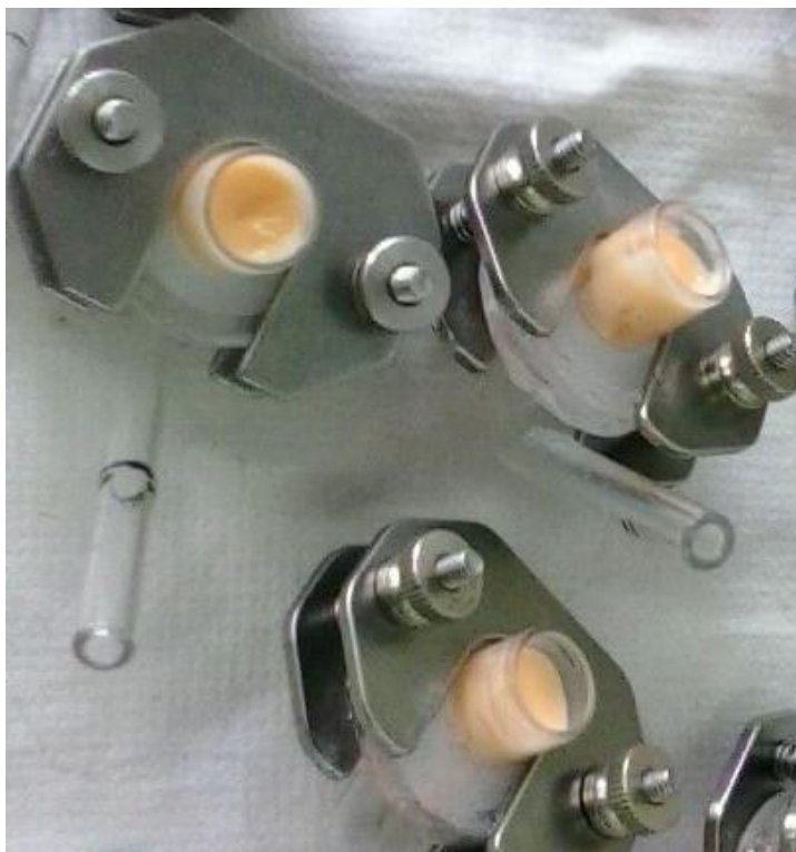
Figure E.7: Photograph of Franz cells, containing the light orange coloured AN-EM and AC-EM formulations
