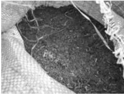
Figure 2-8: Filter material 1: organic medium mixed with Sand
