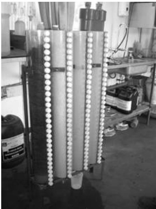
Figure 2-7: Leaching tubes (cylinders) prepared for AMD experimental design
