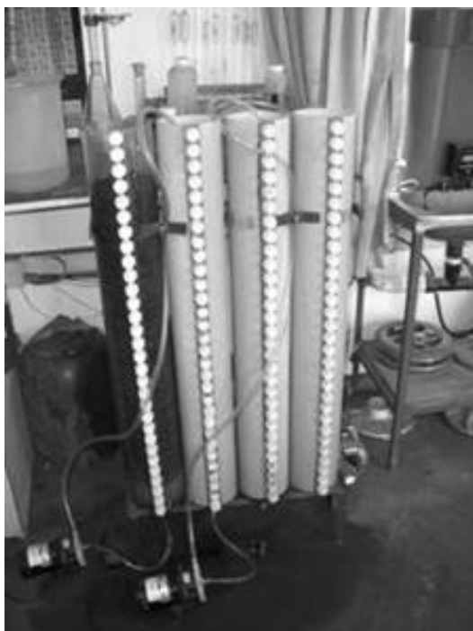
Figure 2-12: Cylinders prepared for AMD test
