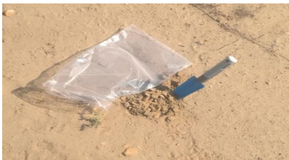
Figure 3. 4: Hand trowel and polyethylene plastic bag for soil sample collection.
