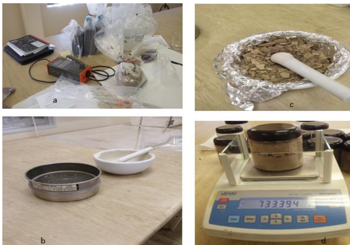
Figure 3. 7: Some of the apparatus used in sample preparation (a) survey meter, (b) 2 mm mesh for sieving, mortar and pestle for pulverising of samples (c) soil sample being pulverised, (d) soil sample sealed in a 500 ml container on a weighing scale.
