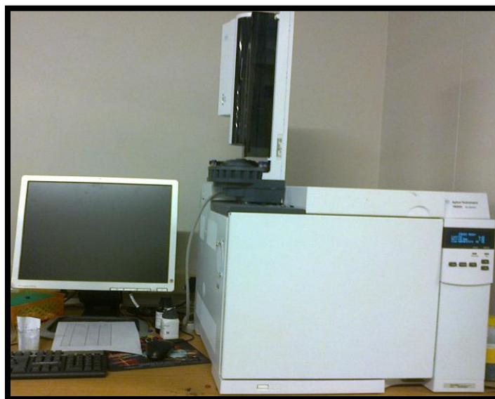
Figure 3-4: GC used to determine fatty acid composition
