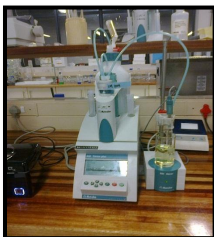
Figure 3-8: Metrohm 848 titrino plus for acid number free fatty acid content determination
