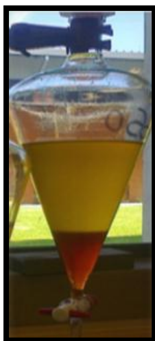
Figure 3-3: Biodiesel separation process
