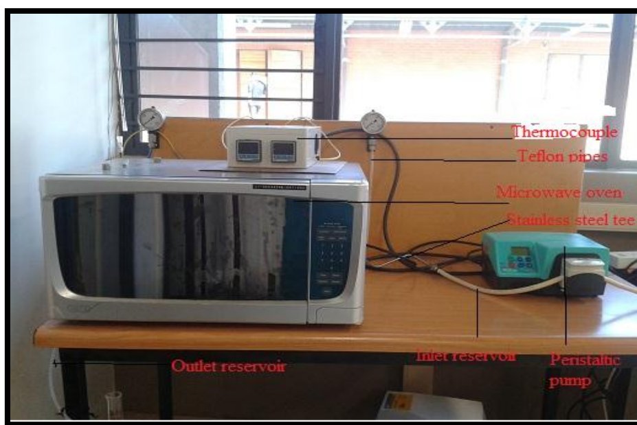
Figure 3-1: Domestic microwave setup for continuous biodiesel production
