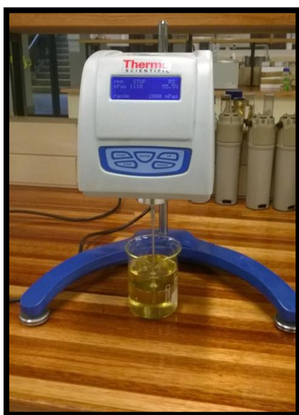
Figure 3-6: A thermo-scientific viscometer used to determine the viscosity of biodiesel
