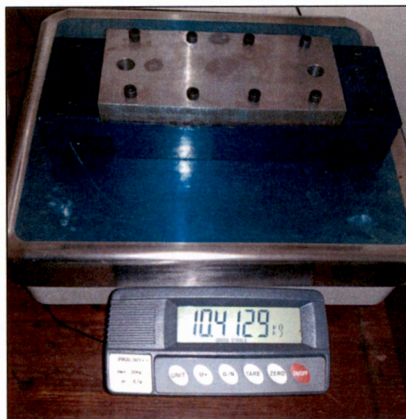
Figure 4.19: Moving mass of Vibration Absorber.
