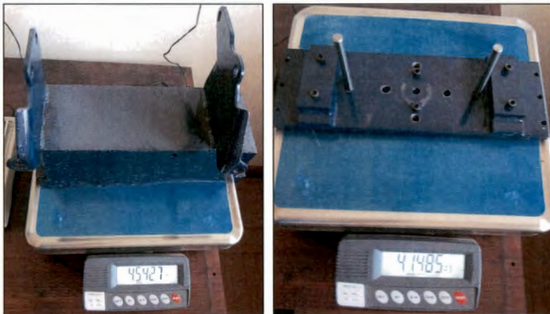
Figure 4.16: Mass of Engine attachment bracket and Absorber basis.
