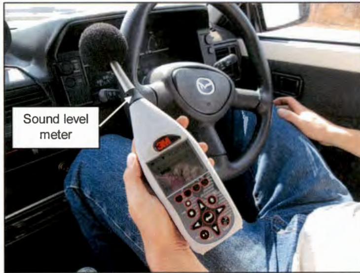
Figure 5.40: 3M SoundPro SE/DL Series Sound Level Meter.
