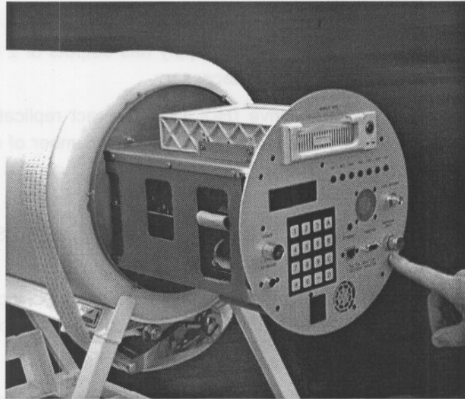
Figure 6.5: The electronics head of the calibration neutron monitor, from the side.
