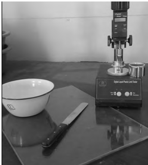
Figure 31: The laboratory equipment to determine plasticity index (Photograph taken by Schmidhuber, 2015, with permission).
