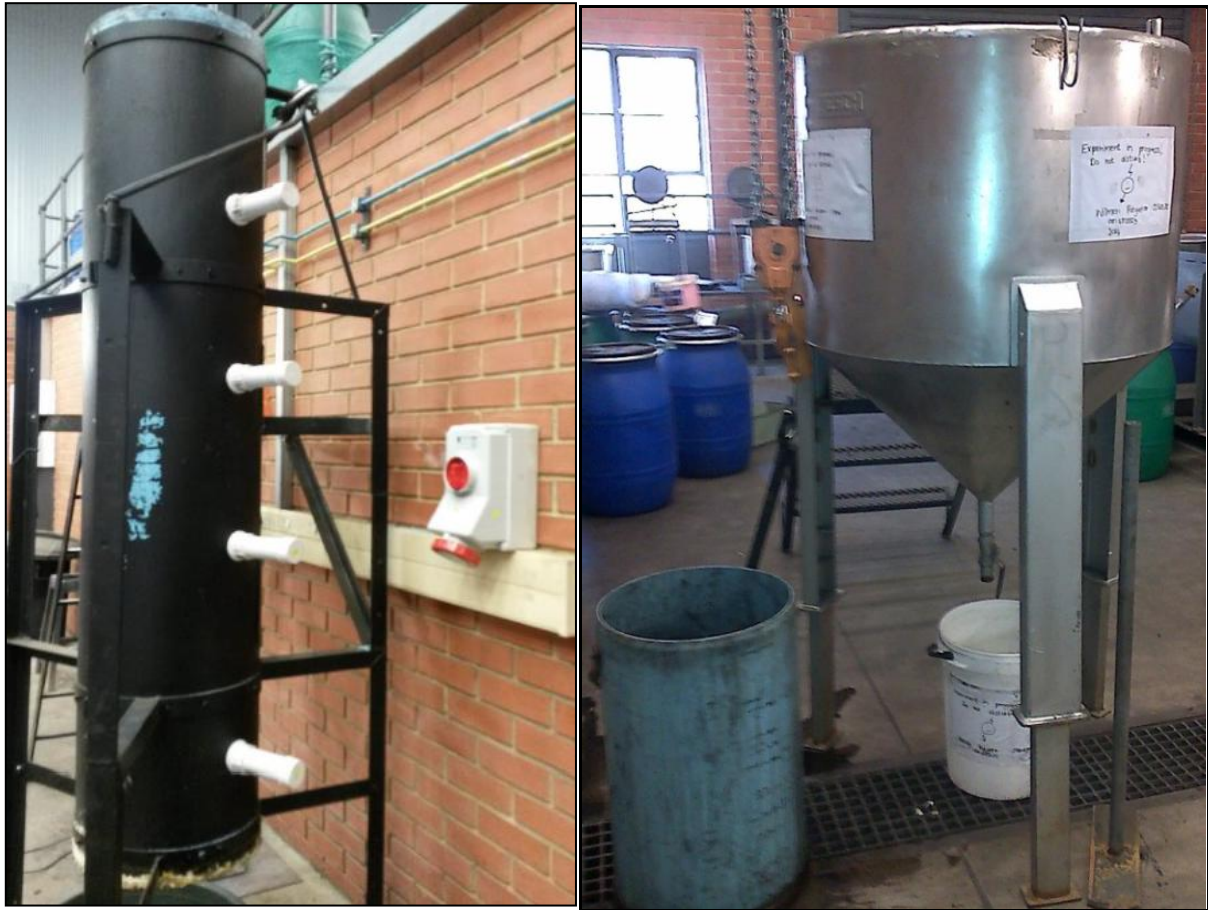
Figure 3.3.1: : Drainage column experimental setup (left: 2m high, right: 0.48 m high)
