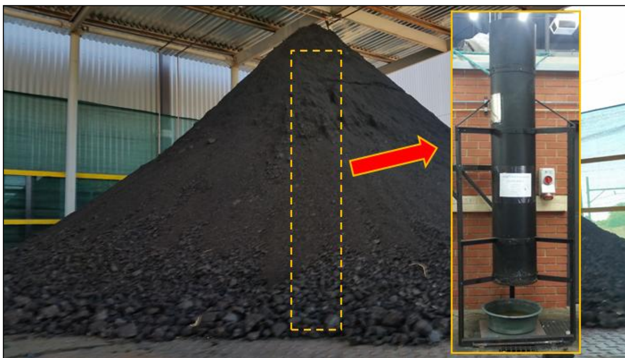
Figure 4.4.6: Illustration of the way by which the drainage column simulates the drainage in a stockpile
