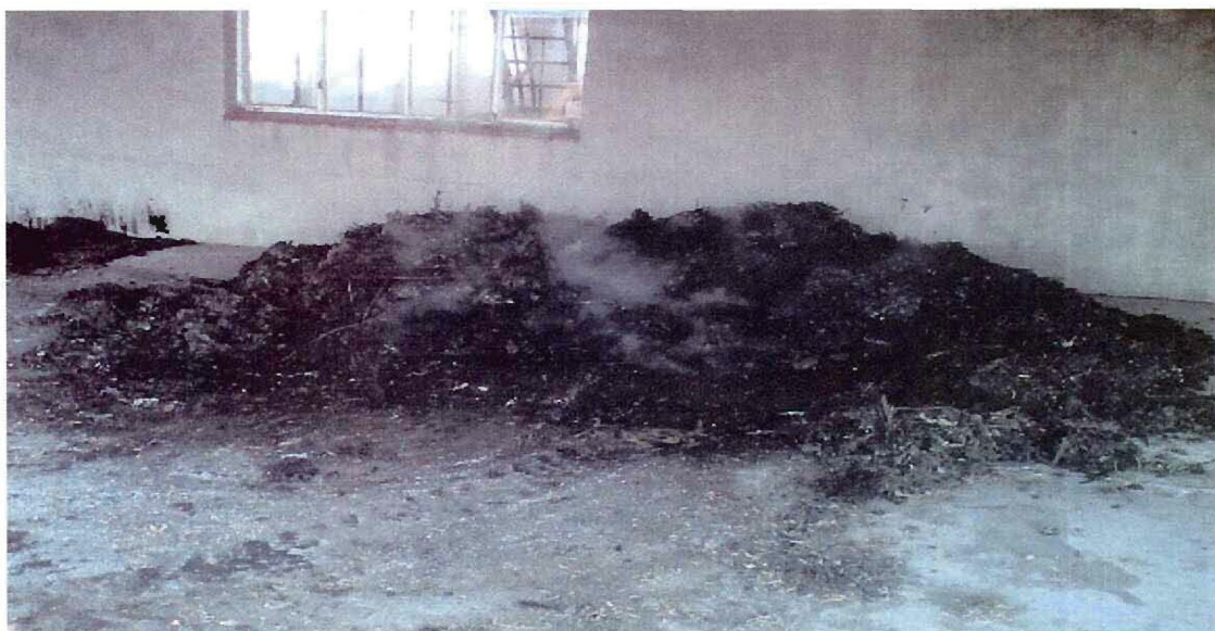
Figure 10: Steam generation during composting as an indication of exothermic reactions during composting of sludge material
