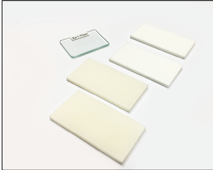
Figure 15: PA2200 and PA2221 samples used for surface roughness tests
