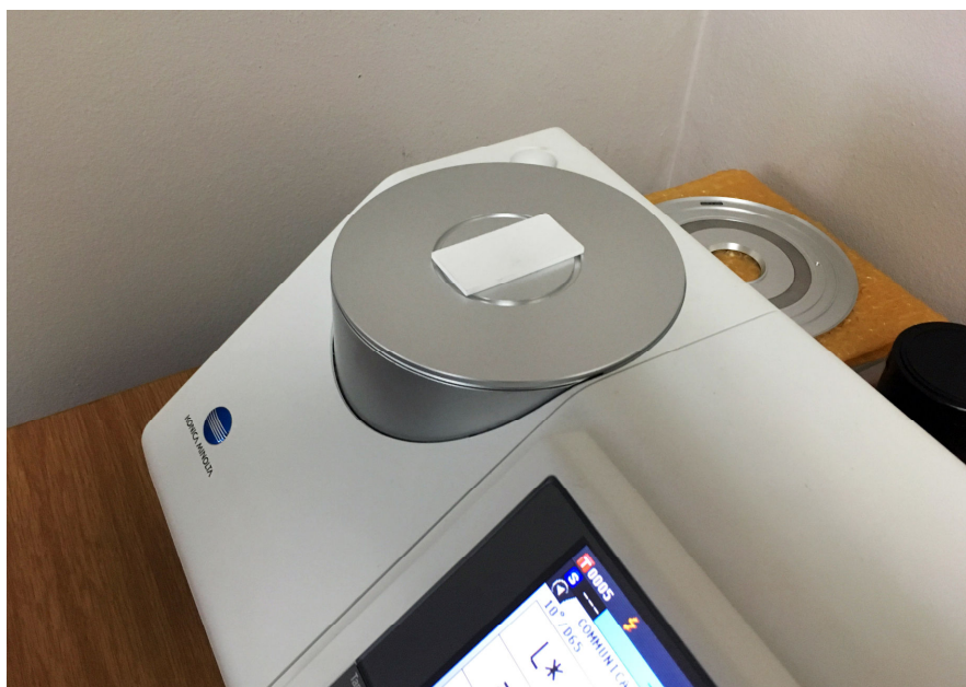
Figure 12: PA2200 sample loaded for analysis
