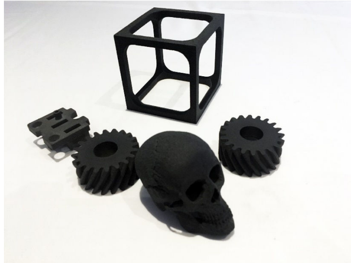
Fig.3. Artefacts sintered in mixed powder
