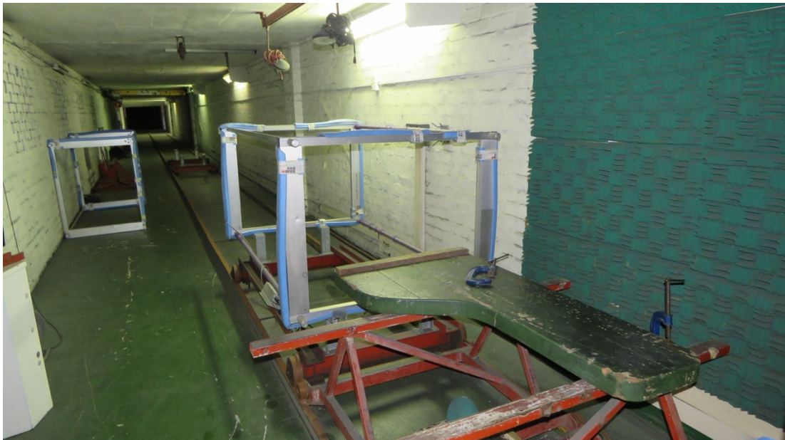
Figure 3. 7: A projectile velocity light barrier used to measure muzzle velocity
