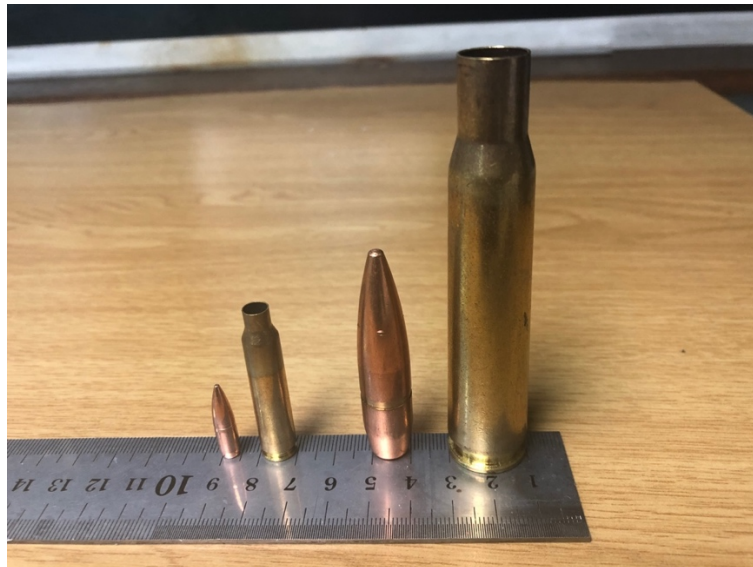
Figure 3. 8: Cartridge case and projectile for 5.56 mm and 12.7 mm bullets respectively
