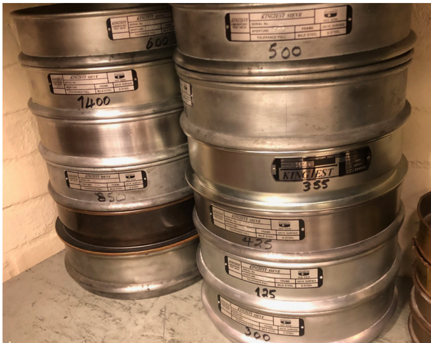
Figure 2: Setup of the sieves to prepare the ball powder samples
