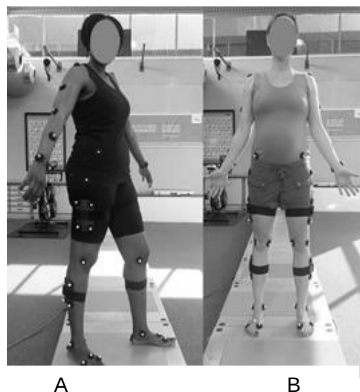
Figure 3.6: Participant ready for data collection with a full-body marker set (A), and static trial (B)
