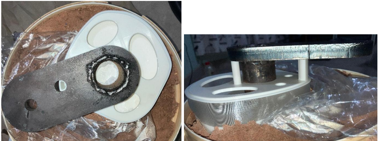
Figure B.14: Stump and Steel Pipe Alignment Jig
