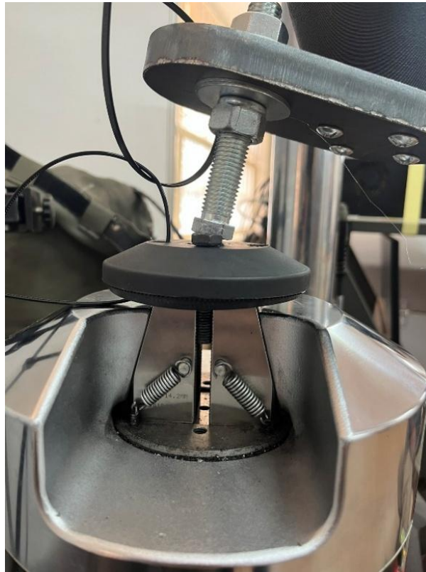
Figure B.16: Clamping condition of the levelling swivel foot
