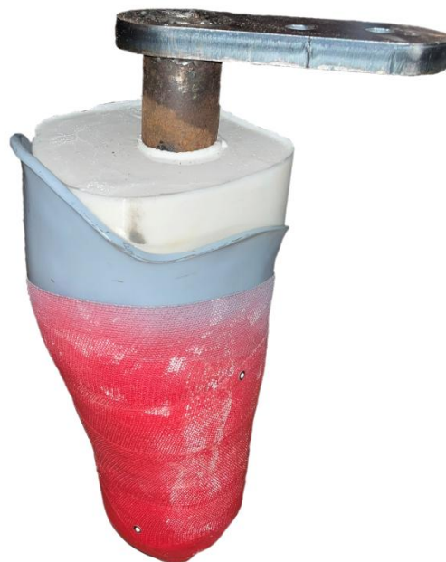
Figure 3.13: Casted Stump fit in scanned TF Check Socket
