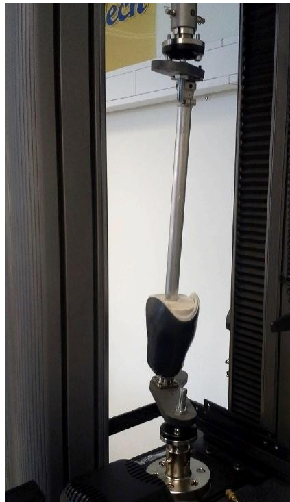
Figure 2.7: Test rig for TT socket in accordance with ISO 10328 (Skoglund, 2015).
