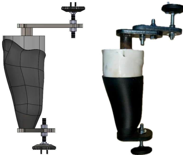
Figure 3.14: Complete Testing Setup (a) CAD Design (b) Modified as built
