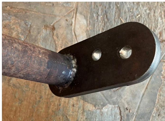
Figure B.13: Steel pipe welded to the top plate
