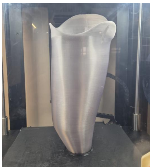
Figure 3.19: Complete PETG TF Socket Prototype
