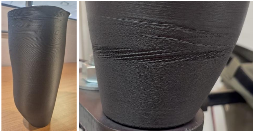
Figure 3.18: ePA-CF 1 specimen's defects (a) Incomplete prototype due to bed adhesion failure (b) Nozzle deposition of blobs on outer walls
