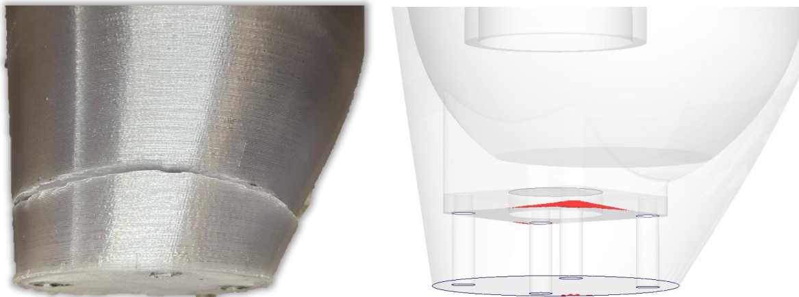
Figure 4.5: a) PETG 1 fracture location external; b) FEA Highest von Mises Stress internal iso-clipping
