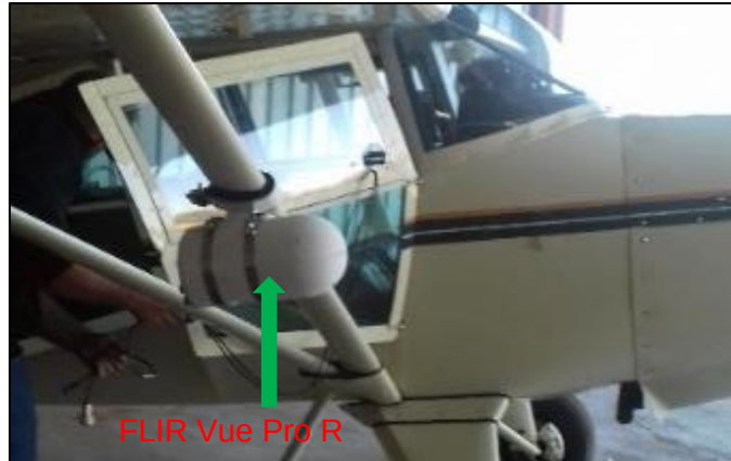
Figure 3.6: FLIR Vue Pro R fixed to an aircraft wing for the acquisition of aerial thermal data
