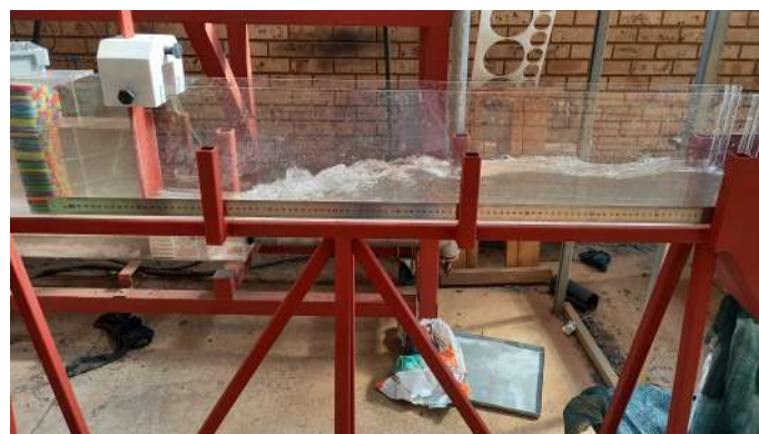
Figure 4: Test bench showing a hydraulic jump in process
