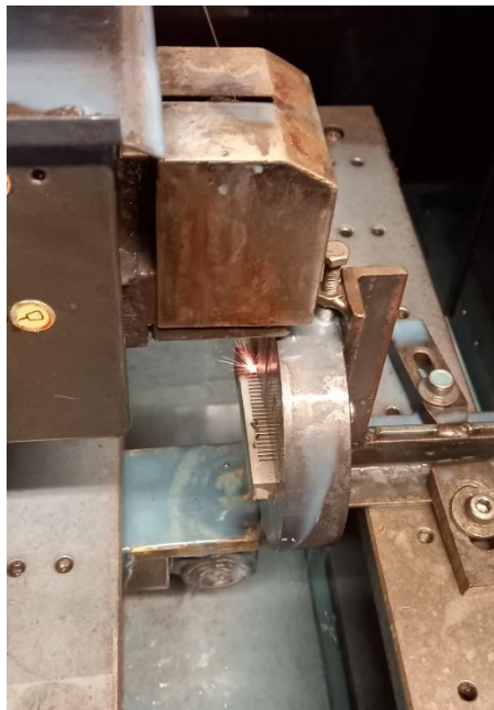
Figure 4-9-Wire electron discharge machine cutting phase.
