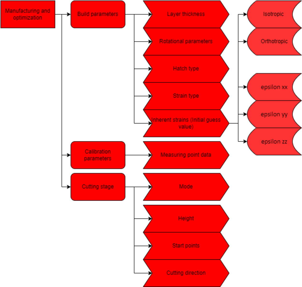
Figure 4-15-Manufacturing and optimisation setup of a simulation procedure
