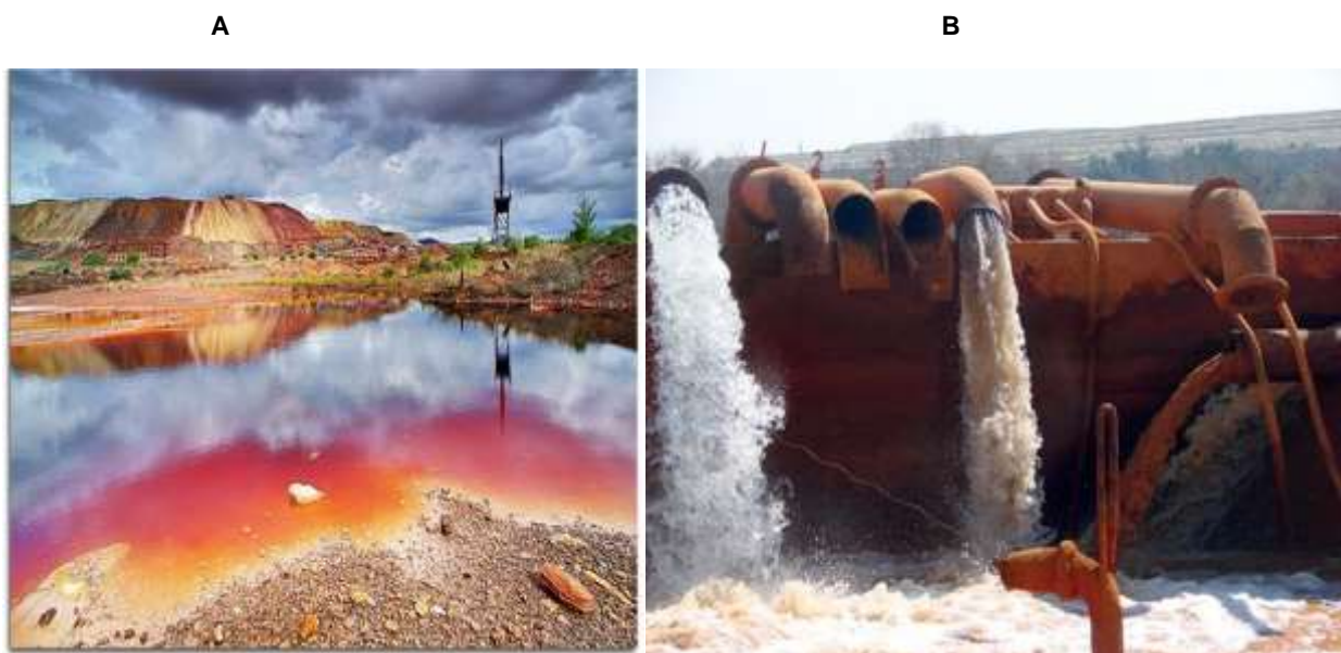
Figure 1-1: AMD seepage from tailings (A) and Pumps at the Grootvlei Mine (B) (WRC, 2011)
