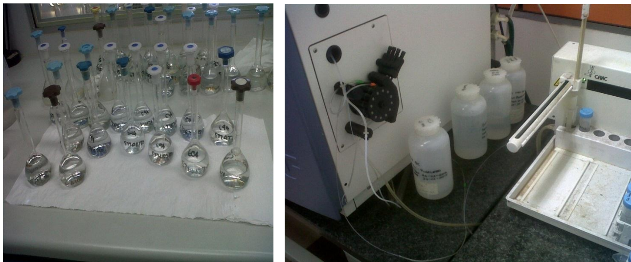
Figure 3-3 Photograph showing the IC standards and QC samples that were prepared (left) and IC analyser pump drawing a sample from the holder into the instrument (right).
