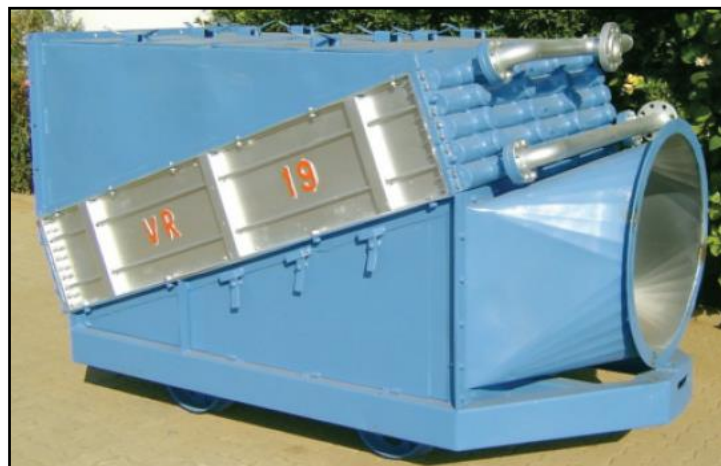
Figure 54: Typical mobile cooling unit 8
