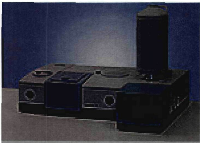
Figure 3.10 The Vertex 70 FT-IR spectrometer coupled to a Raman II (FT-Raman)
