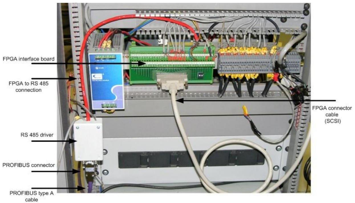
Figure A.3 – RDS motor drive
