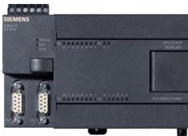
Figure 4.10 – Siemens S7-200 PLC
