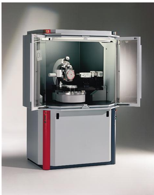
Figure 3.1: A typical XRD apparatus. The apparatus shown in the figure is Bruker's X-ray diffraction D8-Discover instrument.
