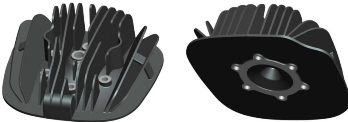
FIGURE 6.2: CYLINDER HEAD FROM A YAMAHA YFS 200 BLASTER.
