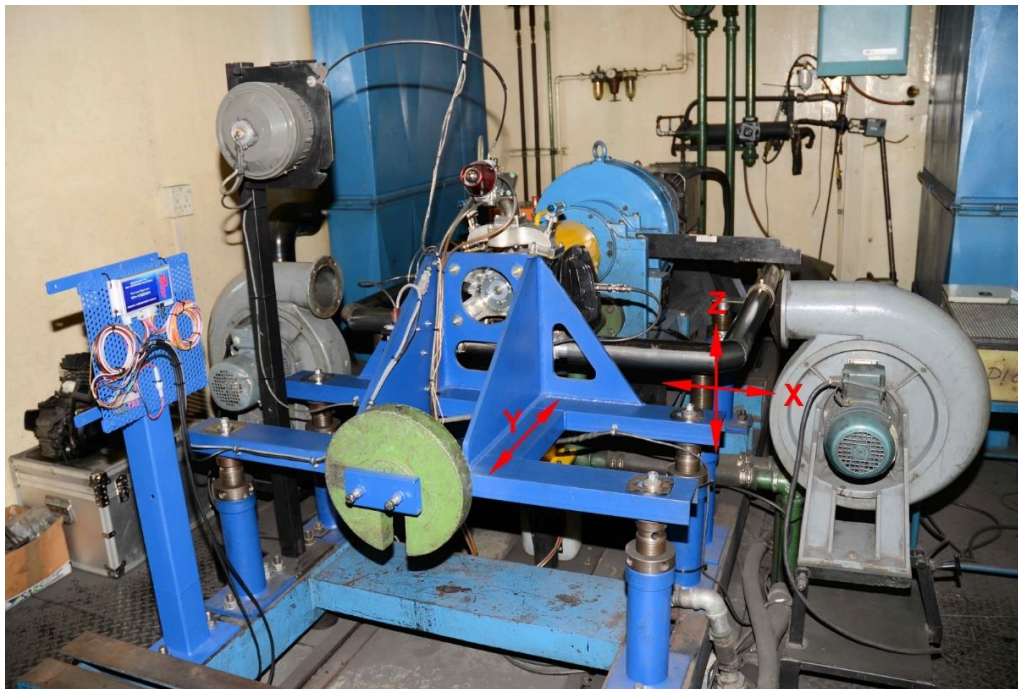
FIGURE 7.2: UAV ENGINE TEST STAND AND INSTALLED PERIPHERAL EQUIPMENT.
