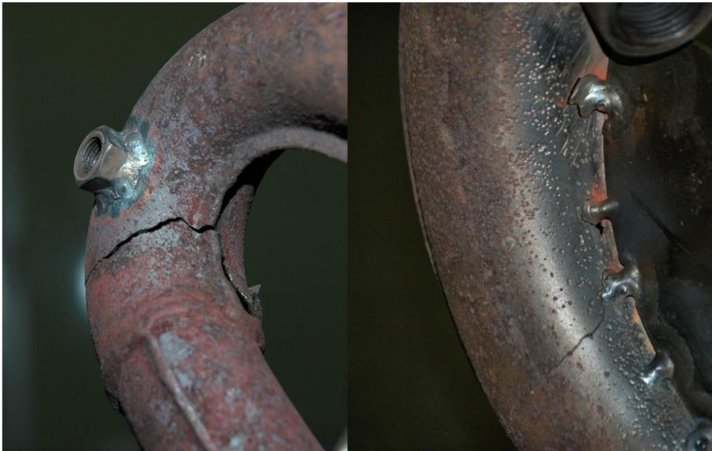
FIGURE 4.10: FIRST AND SECOND EXHAUST FAILURES IN THE VICINITY OF THE EXHAUST PORT.
