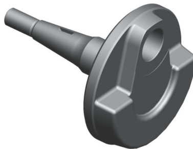
FIGURE 6.5: ONE ORIGINAL OUTER CRANKSHAFT DONOR THROW.
