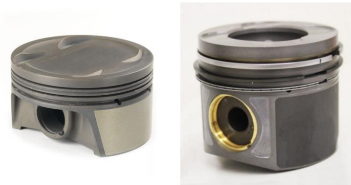
FIGURE 2.17: HONDA F20C, SI PISTON (LEFT) AND BMW M57, CI PISTON (RIGHT). (Courtesy Honda Motor Co., Ltd, Bayerische Motoren Werke AG)
