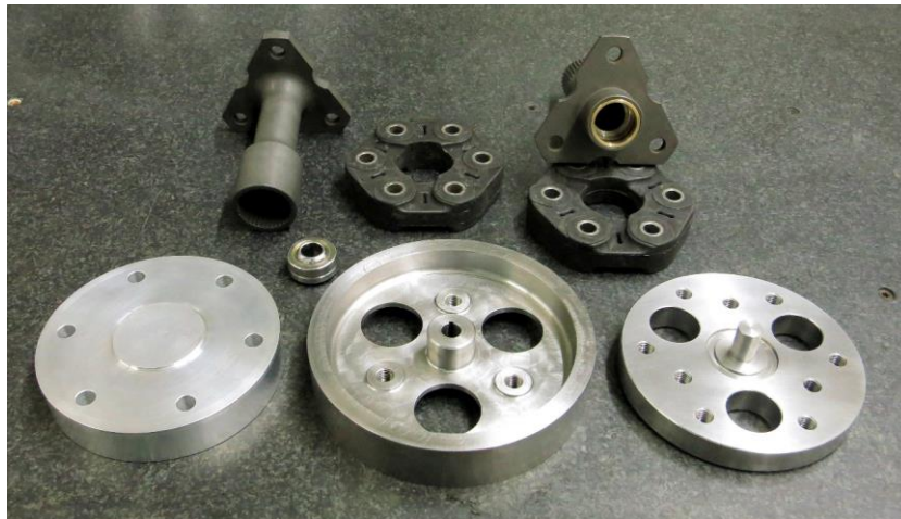
FIGURE 7.12: ALL MANUFACTURED PARTS IN FRONT AND SASOL-SUPPLIED DRIVESHAFT AND TORSIONAL RUBBERS AT THE BACK.
