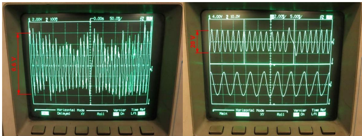
FIGURE 7.6: TRIGGER PULSE VOLTAGE BEFORE (LEFT) AND AFTER REWIRING (RIGHT).
