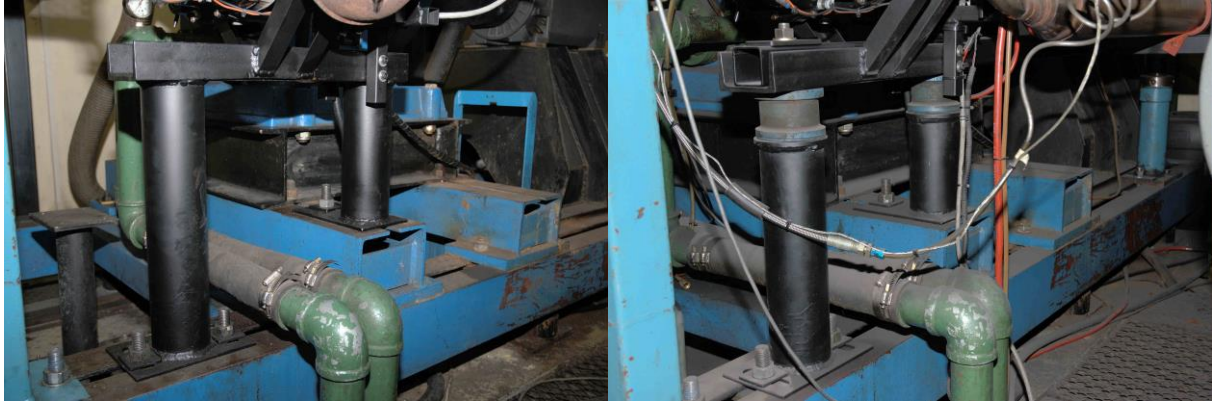
FIGURE 4.9: THE ORIGINAL TUBE PEDESTALS (LEFT) AND (RIGHT) THOSE MODIFIED WITH RUBBER MOUNTS.
