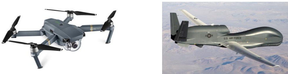
FIGURE 1.1: DJI MAVIC PRO QUADCOPTER (LEFT) AND RQ-4 BLOCK 30 GLOBAL HAWK RECONNAISSANCE AIRCRAFT (RIGHT).
