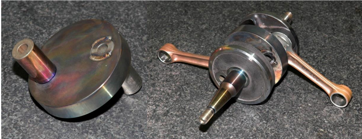
FIGURE 6.7: THE TIG WELDING APPLIED TO THE CRANK PINS ONCE PRESSED INTO THE CENTRAL CRANKSHAFT THROW (LEFT) AND THE ASSEMBLED CRANKSHAFT (RIGHT).
