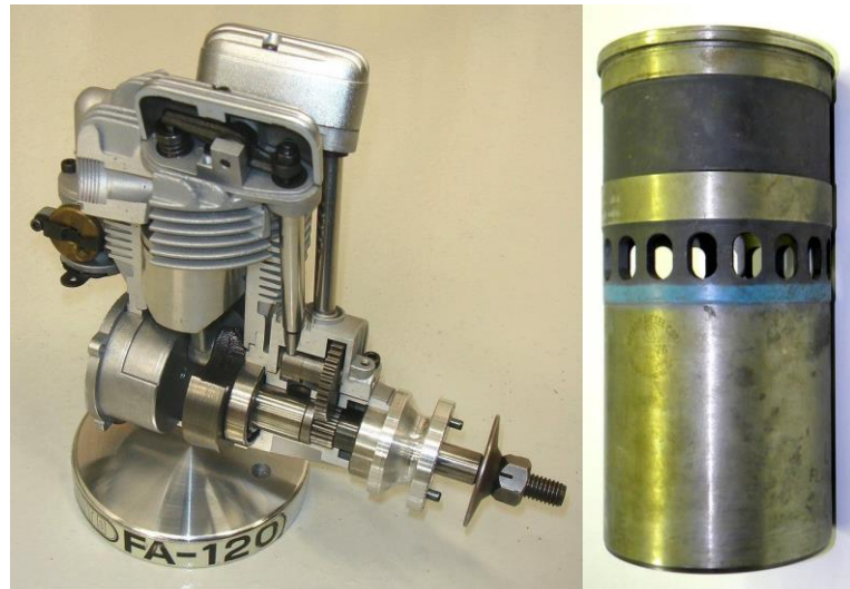
FIGURE 2.4: SAITO FA-120 FOUR-STROKE ENGINE (LEFT) AND DETROIT DIESEL 8V92 TWO-STROKE SLEEVE (RIGHT).
