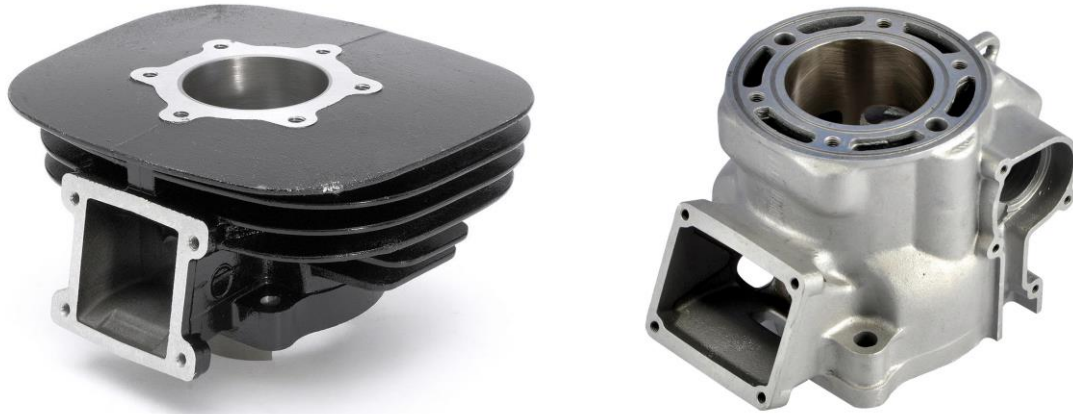
FIGURE 2.14: YAMAHA YFS 200 BLASTER AIR-COOLED CYLINDER (LEFT) AND A YAMAHA YZ 250 LIQUID-COOLED CYLINDER (RIGHT).
