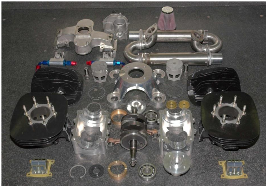
FIGURE 6.21: ENGINE COMPONENTS AND SYSTEMS OF THE UAV ENGINE.
