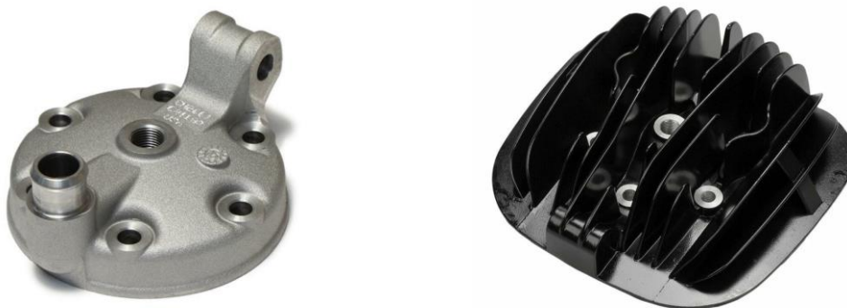
FIGURE 2.22: YAMAHA YZ 250 LIQUID-COOLED CYLINDER HEAD (LEFT) AND YAMAHA YFS 200 AIR-COOLED CYLINDER HEAD (RIGHT) FOR TWO-STROKE ENGINES.
