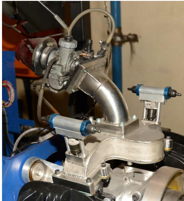
FIGURE 7.7: MIKUNI VM26SS CARBURETTOR AND INTAKE RUNNER BOLTED TO THE CENTRAL PLENUM.
