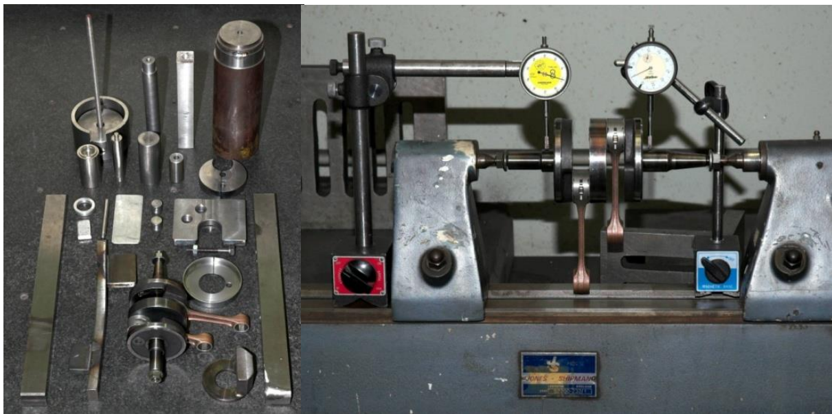
FIGURE 6.9: TOOLING AND JIGS FOR ASSEMBLING AND ALIGNING THE CRANKSHAFT (LEFT) AND ALIGNMENT OF THE CRANKSHAFT CHECKED BETWEEN CENTRES BY DIAL GAUGES (RIGHT).
