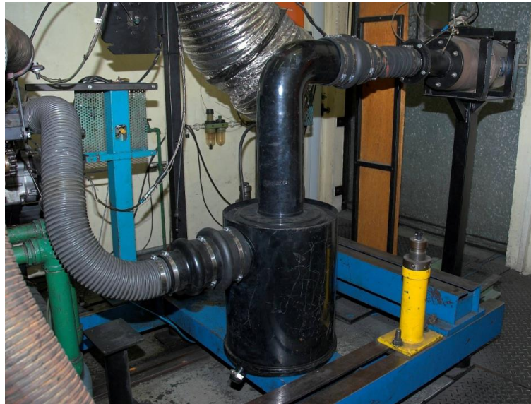
FIGURE 4.11: AIR FLOW METER WITH IN-LINE TRUCK FILTER ATTACHED.
