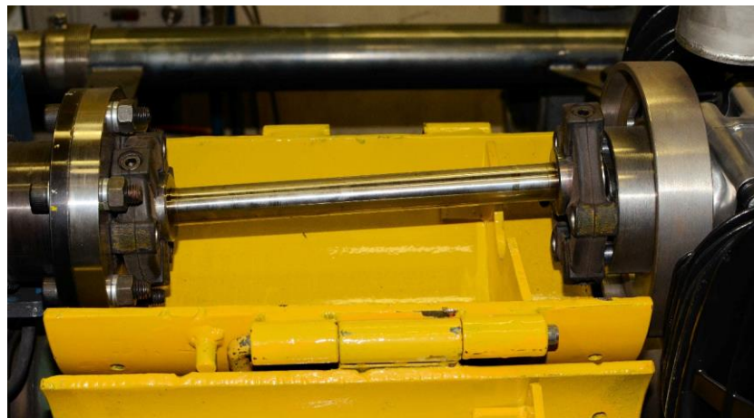
FIGURE 7.9: FAILED CENTAFLEX TORSIONAL DRIVESHAFT.
