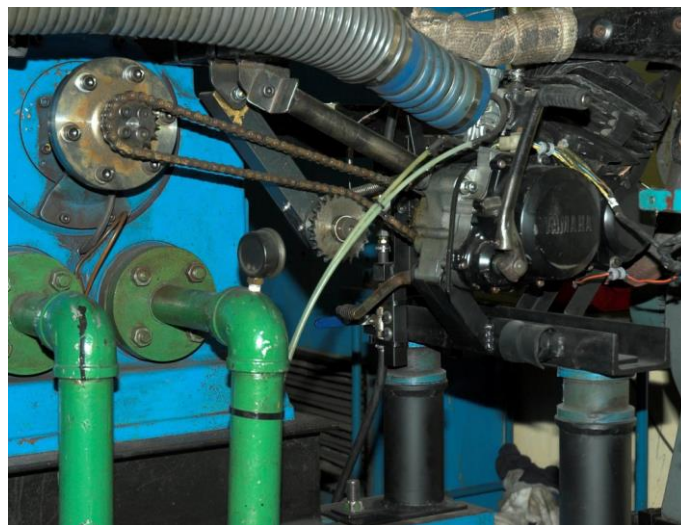
FIGURE 4.4: TEST ENGINE MOUNTED TO TEST BED AND CHAIN DRIVE COUPLING.
