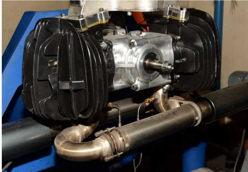
FIGURE 7.4: EXPERIMENTAL ENGINE TEST CELL EXHAUST SYSTEM.
