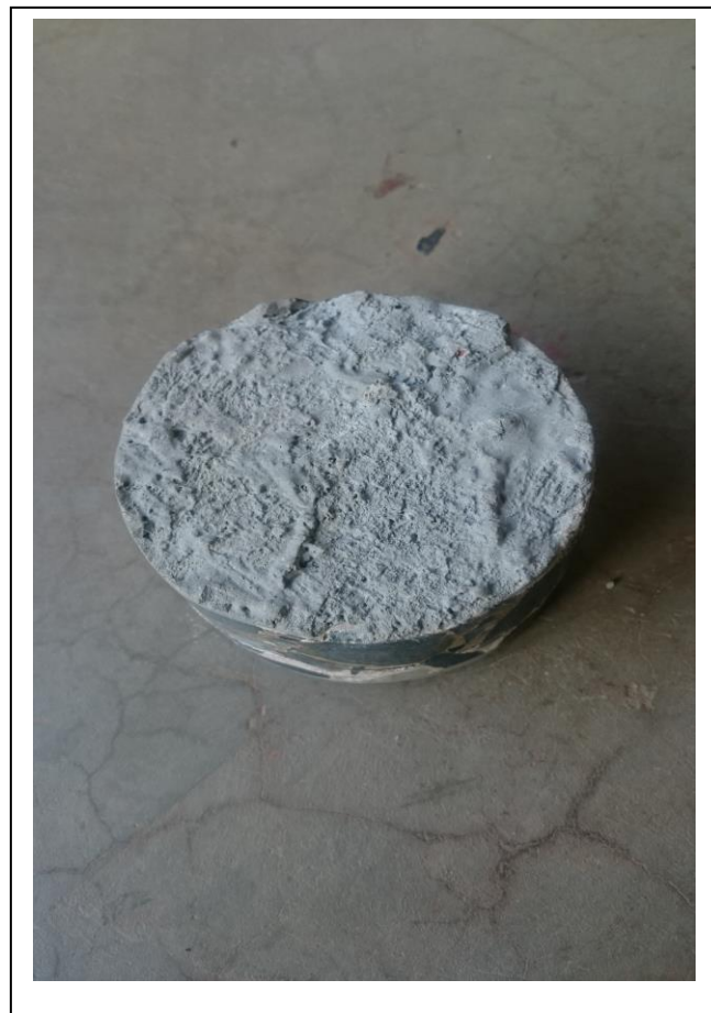
Figure 14: Photo of CEM II concrete with sulphur based coating, illustrating the variation in coating thickness
