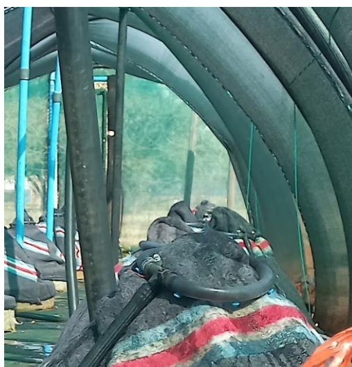
Figure 4.1: Irrigation water outlet used to maintain relative humidity in the treatments.
