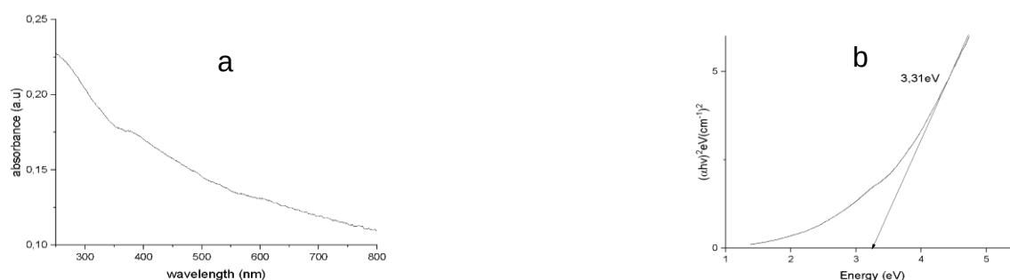
Figure 3.6: (a) UV-vis absorption peak and (b) its corresponding Tauc plot for the band gap estimation
