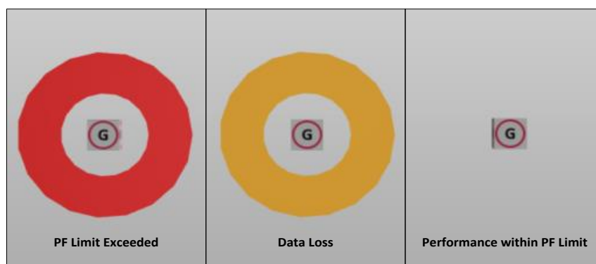
Figure 43: PTB notification system – instrumentation box
