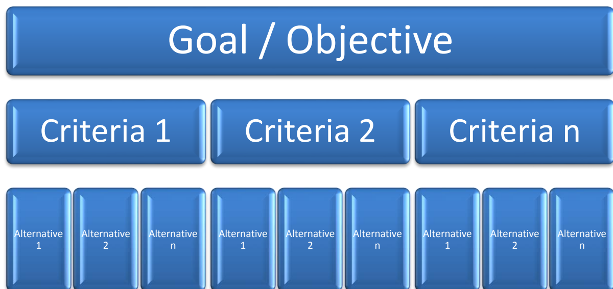
Figure 1-2: Generic Hierarchic Structure of the Analytical Hierarchy Process
