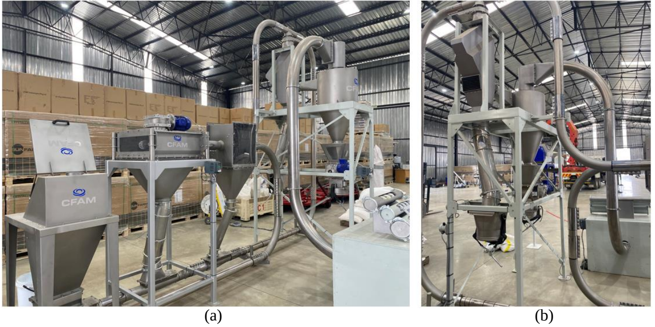
Figure 3: Grain aspiration system experimental setup
