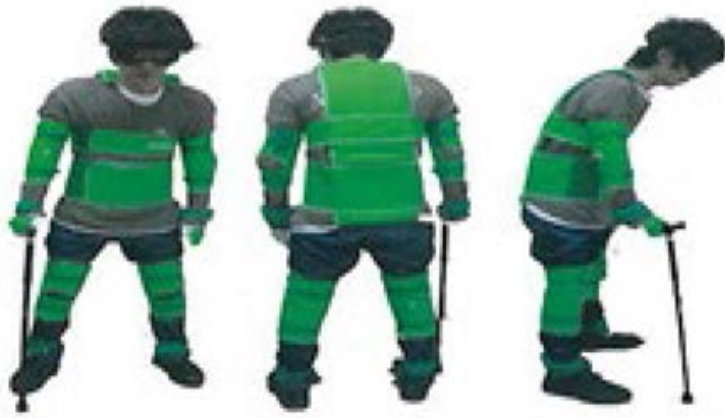
Figure 5-3 Example of ageing simulation equipment (Hong, 2015:4)
