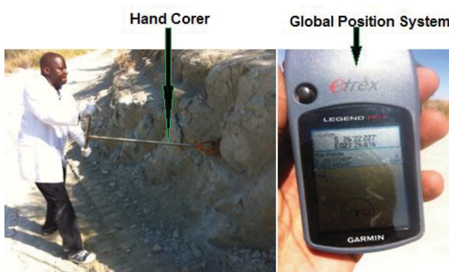
Figure 3.4: Hand Corer and Global Positioning System (GPS) used during Sampling
