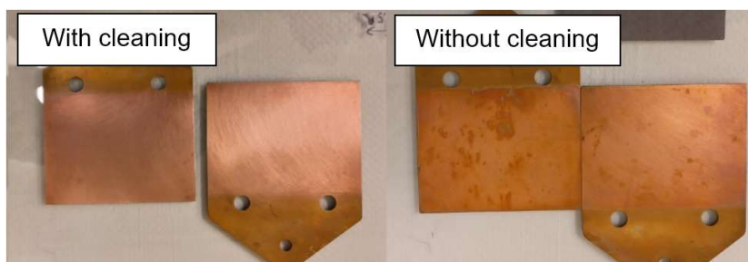
Figure 6.3: Copper current collectors with and without routine surface cleaning.
