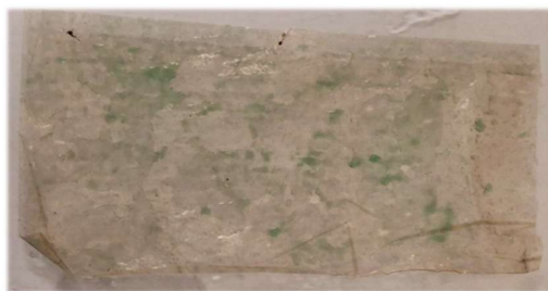
Figure B8: Photograph of fibre mat composite membrane PPFS-D with electrolyte trapped in-between delaminated polymer layers.
