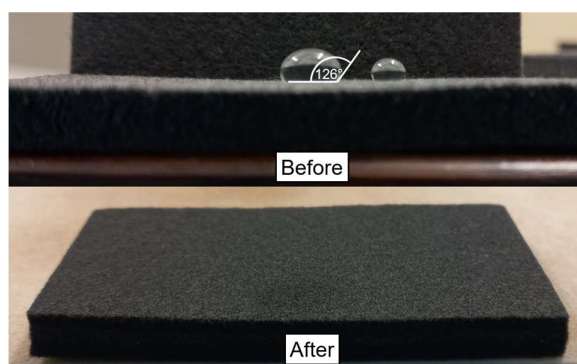
Figure A4: Wettability of CT GF065 graphite felt electrodes before and after thermal treatment.
