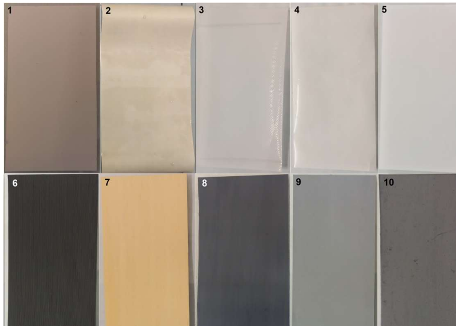
Figure A1: Photographs of new cut MPS samples: (1) EW-200, (2) EW-200 Gen 2.2, (3) C-5550, (4) C-3401, (5) C-2340, (6) Breathtech, (7) DARAK 2000, (8) VANADion-20, (9) AA175 and (10) AA900.
