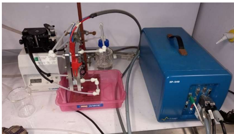
Figure 6.1: Initial ICFB test station (V1) design.
