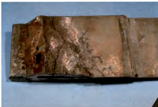
Fig. 9: Stress corrosion cracking
