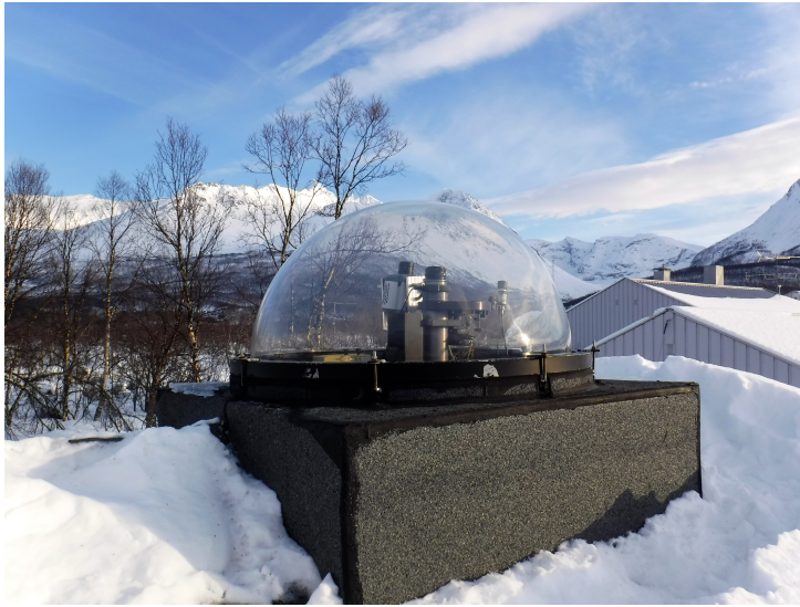
Figure 3.1: Camera setup for the 2016 campaign. On the left-hand side is an iXon-888 EMCCD pointing into the magnetic zenith, fitted with a 427.8 nm filter. The camera in the middle is an ALTA-U47 back-illuminated full frame megapixel CCD pointing into the local zenith, fitted with a 844.6 nm filter. On the right-hand side is a TV imager camera pointing into the local zenith. Image was taken by the author during the 2016 campaign.
