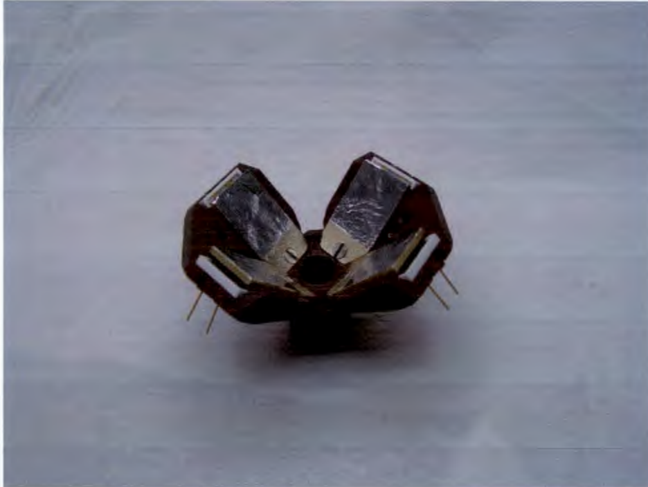
Fig.3.3 Si PIN photodiodes detector at MRG NMP Chamber, iThemba LABS
