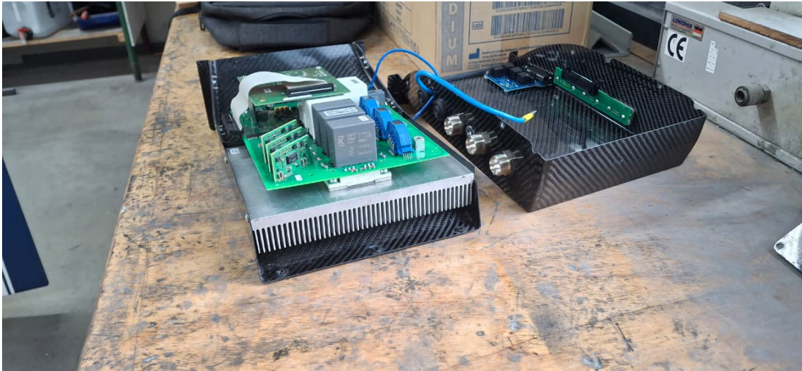
Figure 1.4: Motor controller heat sink and internal thermal path.
