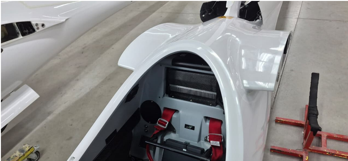
Figure 3.7: Motor-controller packaging inside the fuselage (cockpit-side view)
