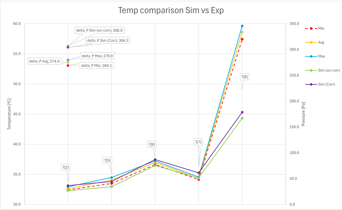
Figure A.18: Comparison of measured and simulated temperatures and pressure drop (corrected for altitude)
