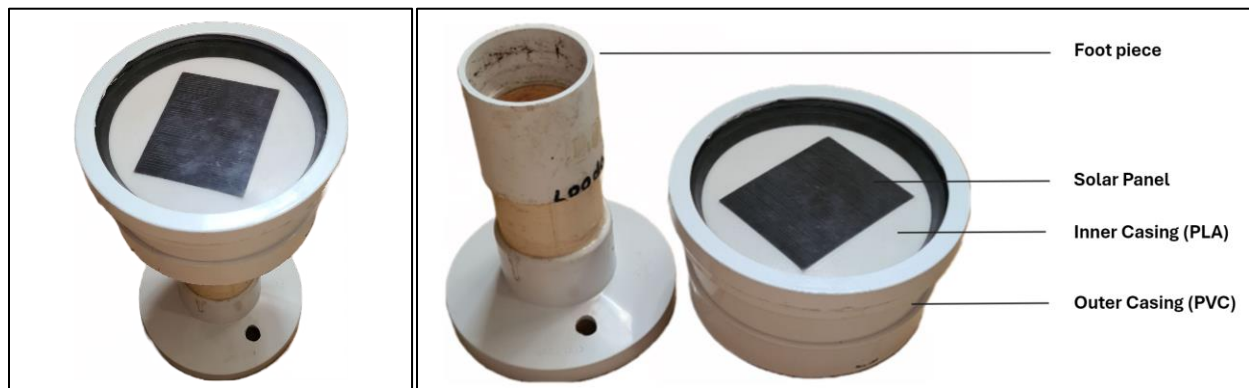
Figure 4-5: The implemented in-road casing assembled (left), with a separate foot piece (right)
