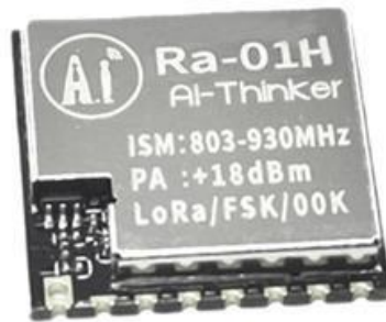
Figure 3-10: The Ra-01H module housing the SX1276 LoRa chip [47]
