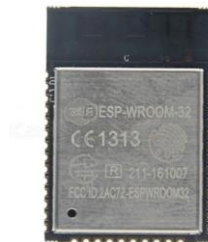
Figure 3-12: The ESP32-WROOM 32-E modules [49]
