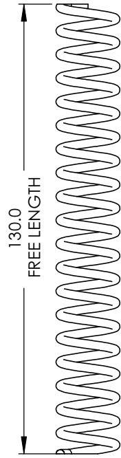
⑬ HARD SPRING QUANTITY: 1 MATERIAL: MUSIC WIRE 2.5MM SPRING RATE: 5.25 N/MM
