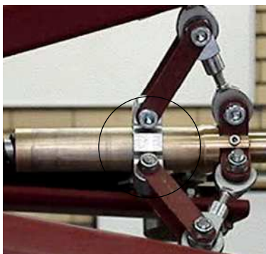
Figure 7.8 Friction between synchronisation bush and connector
