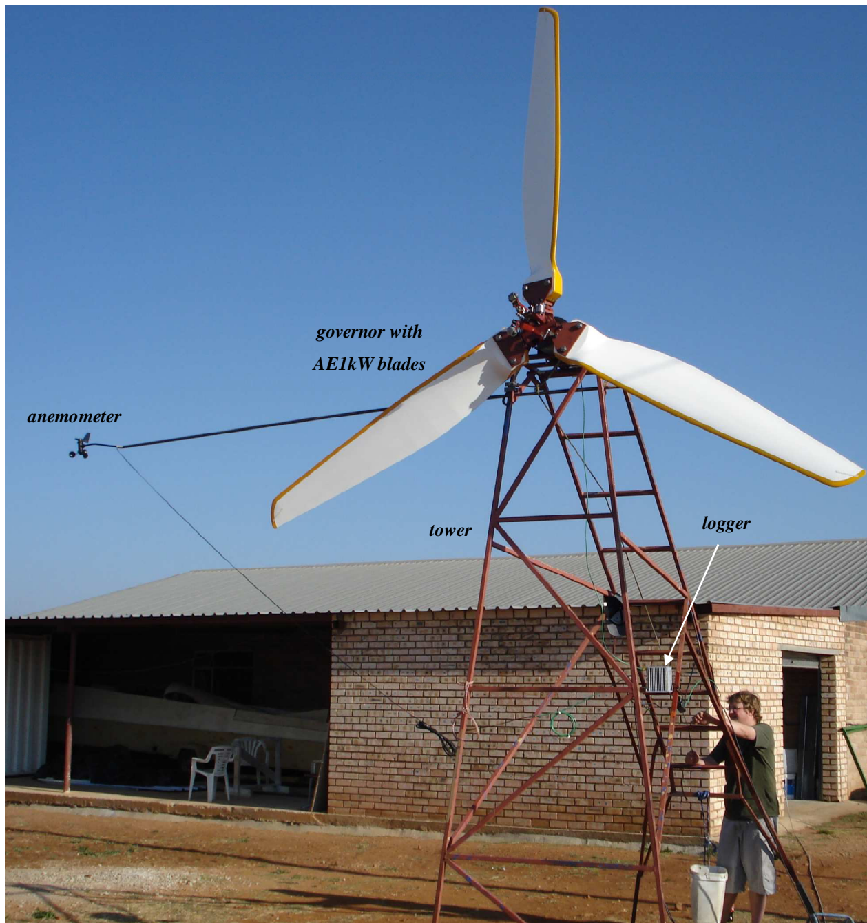
Figure 7.13 Experimental setup of the governor prototype with the AE1kW blades
