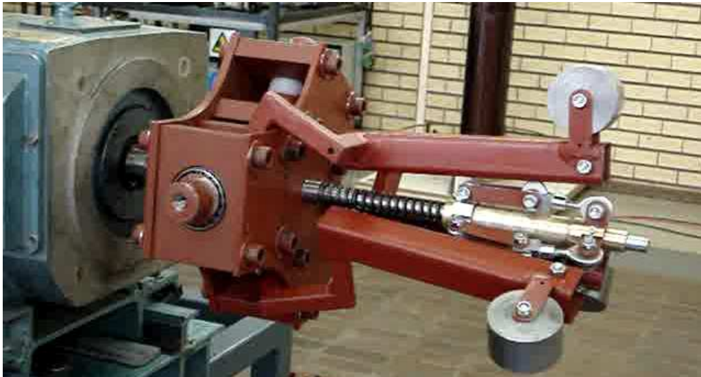
Figure 7.1 Initial test setup with the governor prototype in the start-up position without blades
