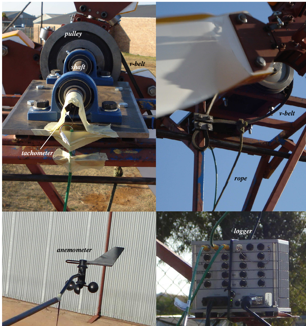
Figure 7.14 Experimental setup of the governor prototype with the AE1kW blades
