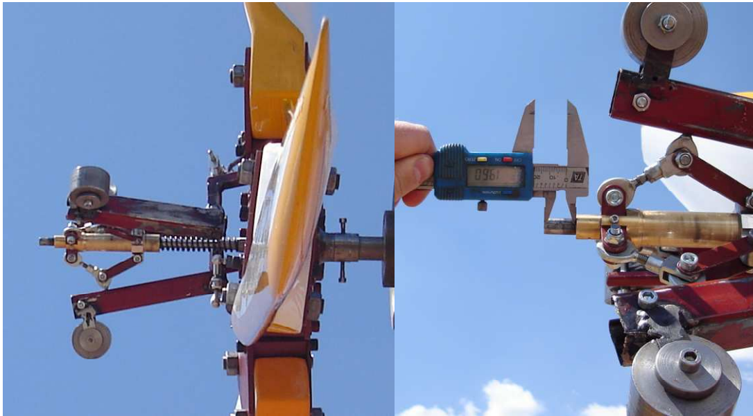
Figure 7.29 Improved start-up position of the modified prototype
