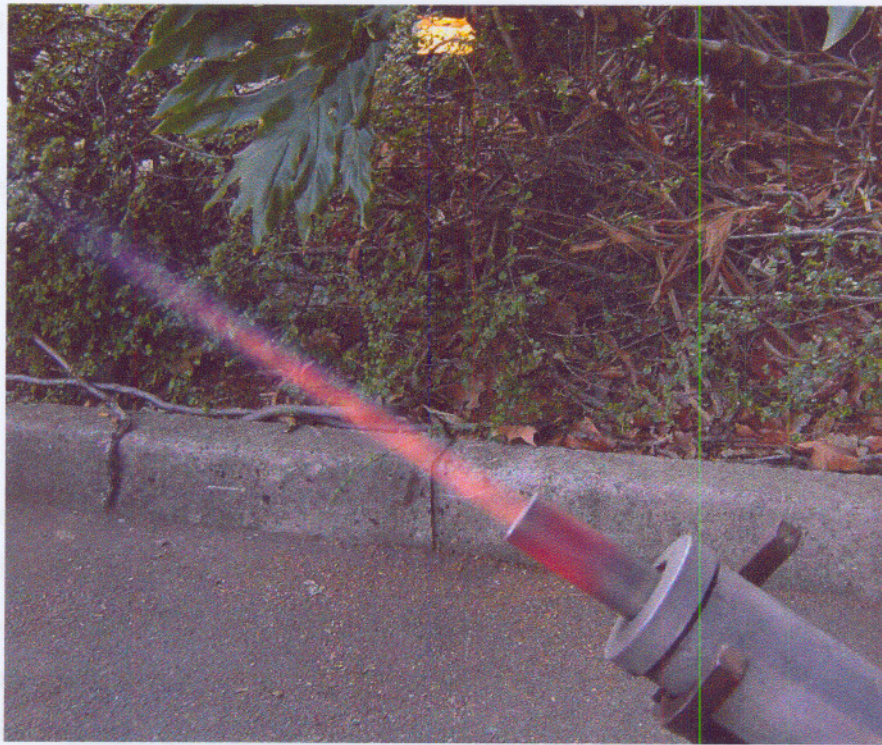
Figure 7.4. WC nozzle colour during normal operating conditions
