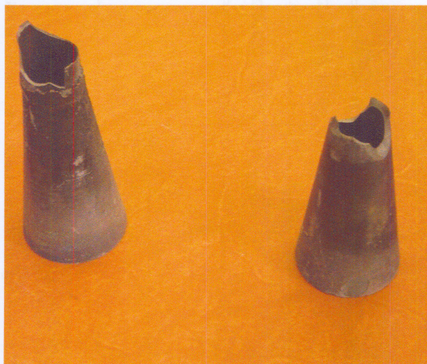
Figure B.6 WC nozzles with the 50 and 70 mm long diverging sections after tests
