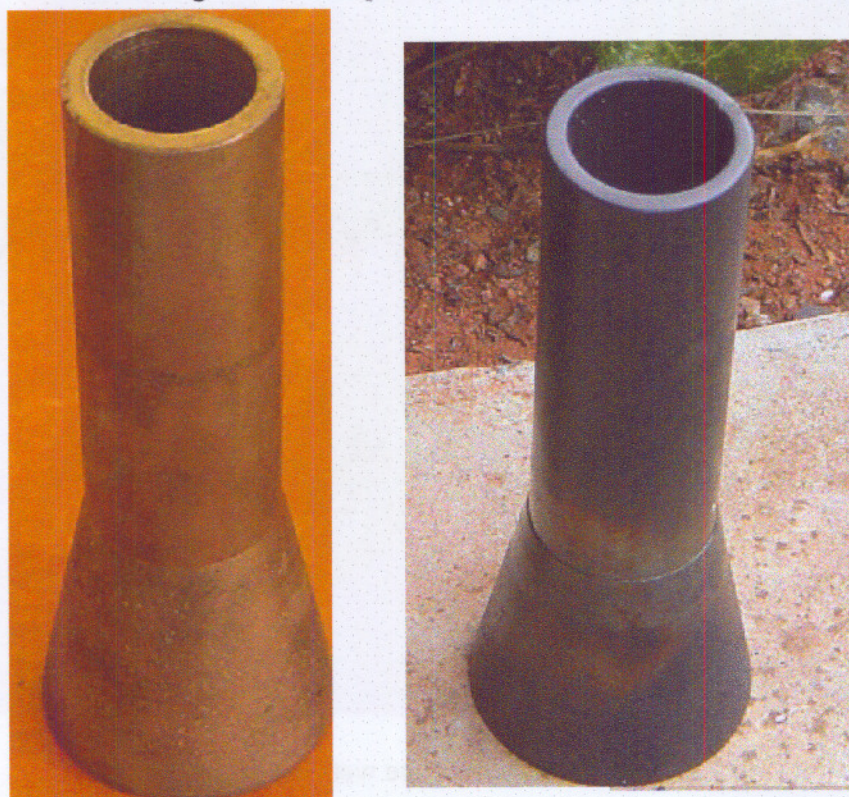
Figure B.8 WC nozzles with the 70 mm long diverging sections before and after tests
