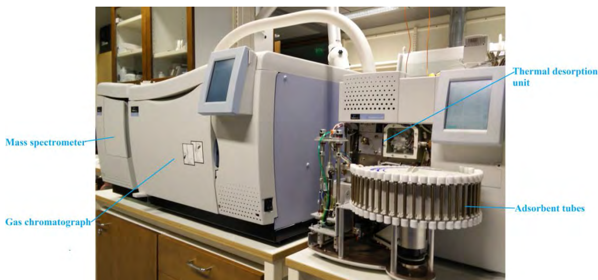
Figure 3-7: Thermal desorption instrument connected to a gas chromatograph and a mass selective detector
