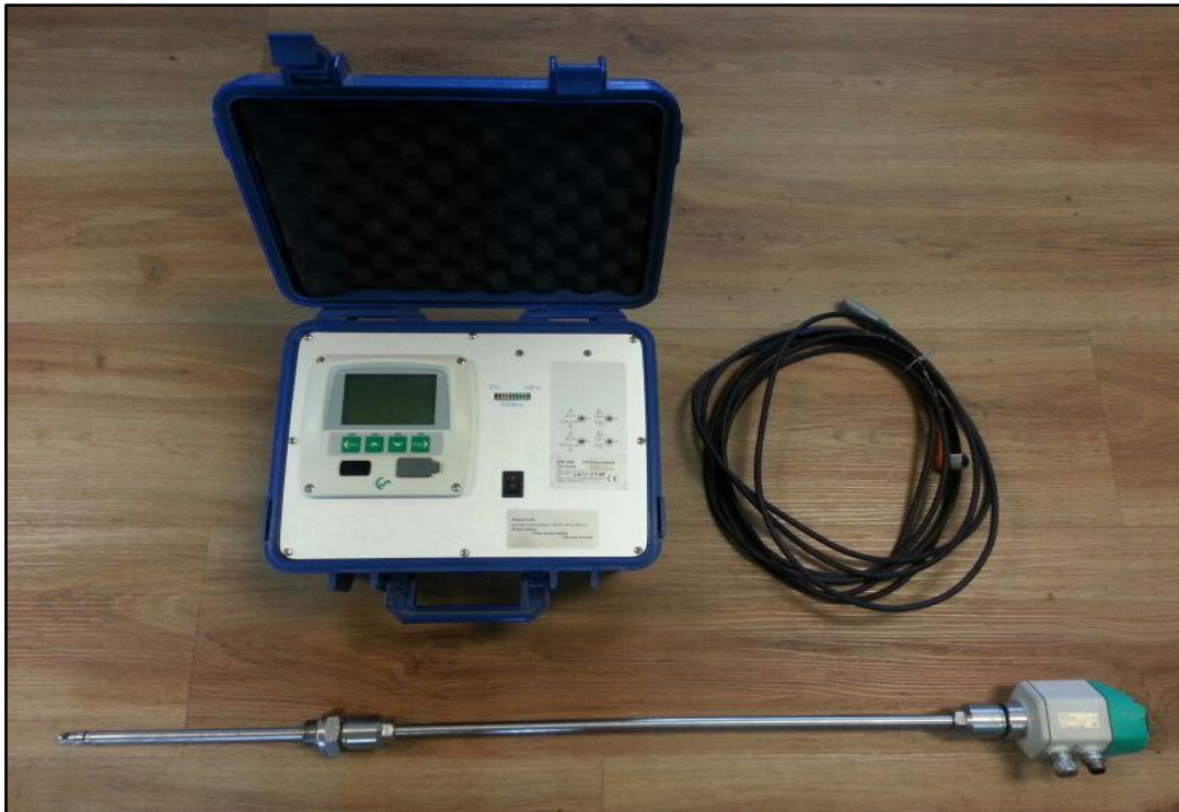
Figure 32: Portable flow meter 12
