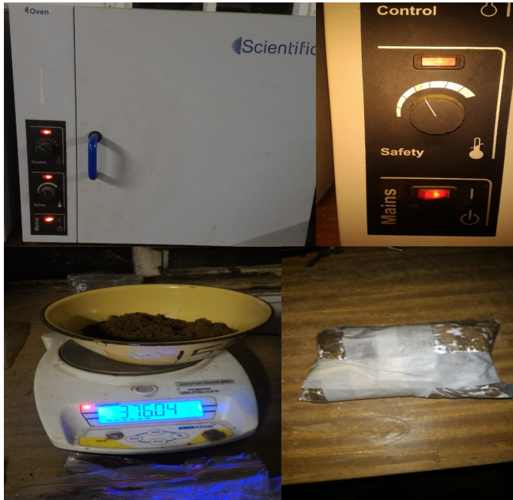
Figure 7: Laboratory setup for sample weighing and drying.
