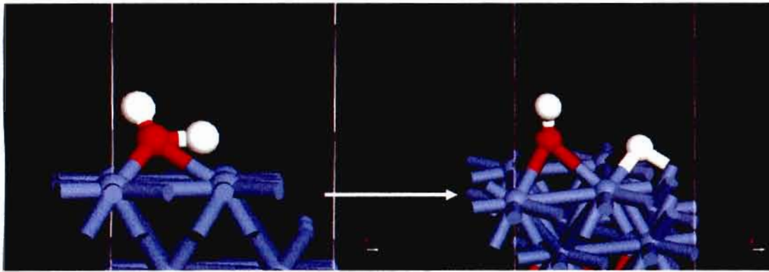
Figure 12-7: Structure of H 2 O molecular (O-red, H-white) adsorption on Fe(110) tilted on the surface, showing dissociation of water on Fe(110) surface and co-adsorption of OH and H.
