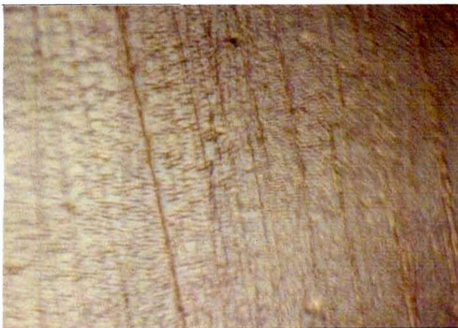
Figure 8-7: FTIR microscope image of adsorbed BATE on warm water treated LCAK surface
