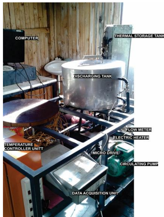
Figure 5.1: A photograph of the main components of the experimental thermal energy storage system [20].
