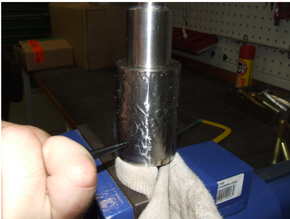
Figure C.1: Glue between rotor laminations and PM
