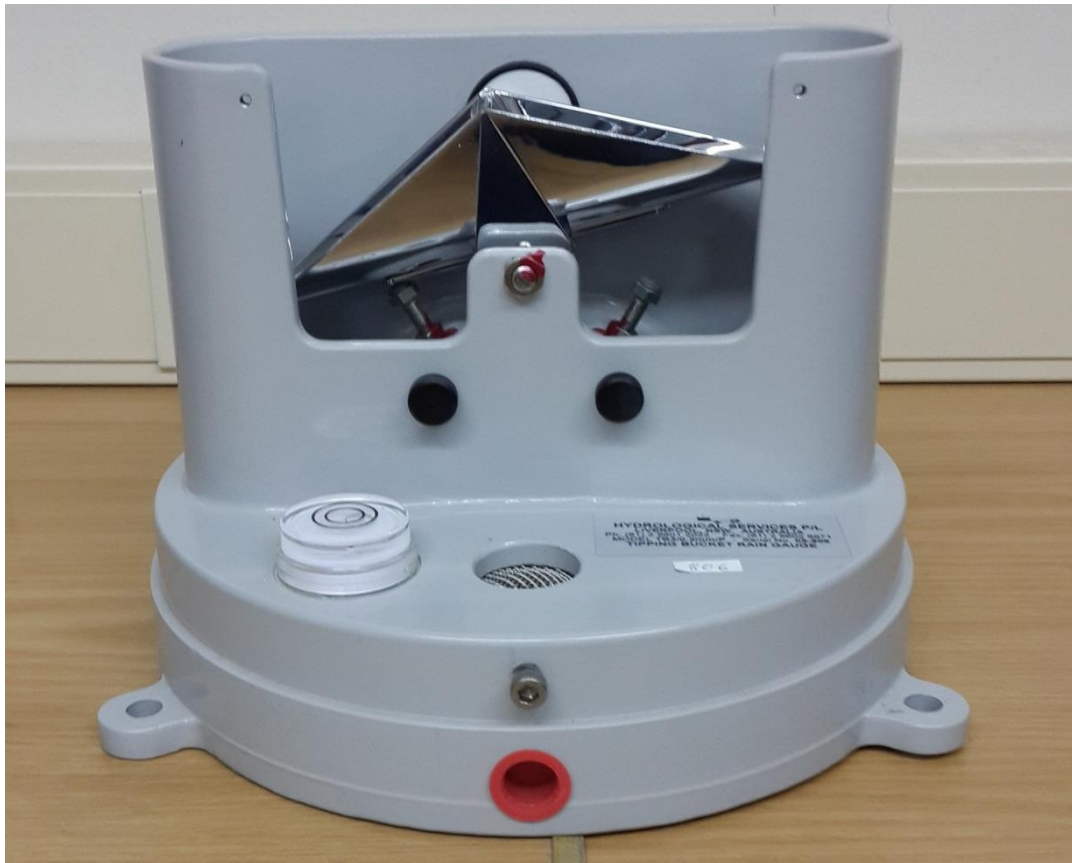
Figure 2-6: The measuring system of the TB 3 tipping bucket rain gauge.
