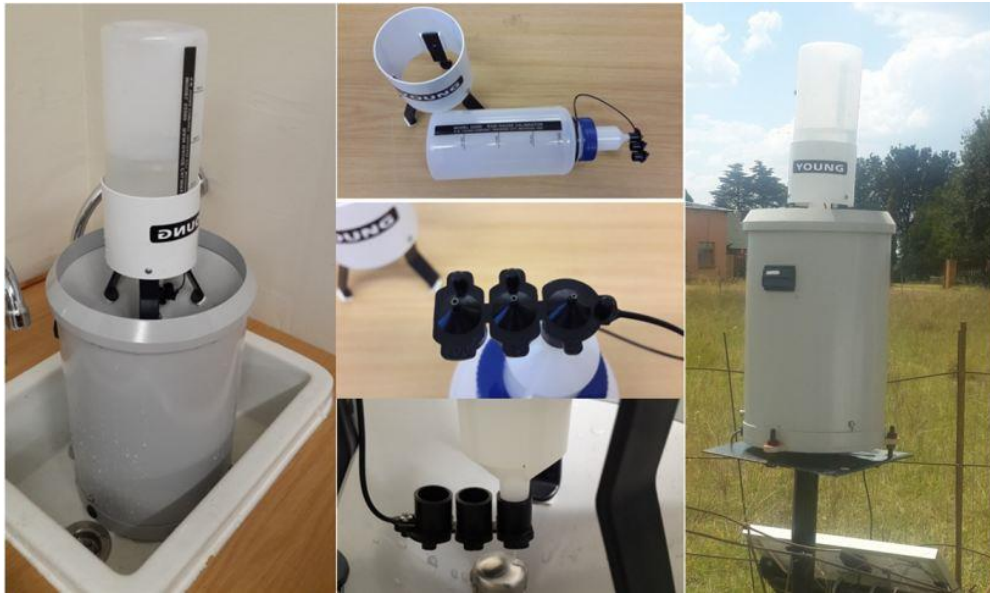
Figure 2-13: Laboratory and field calibration of rain gauges. The gauge is calibrated before deployment in the lab (left photo). The calibrator has three nozzles to simulate different rain rates (Middle photo's). The gauge being calibrated in the field (right photo).
