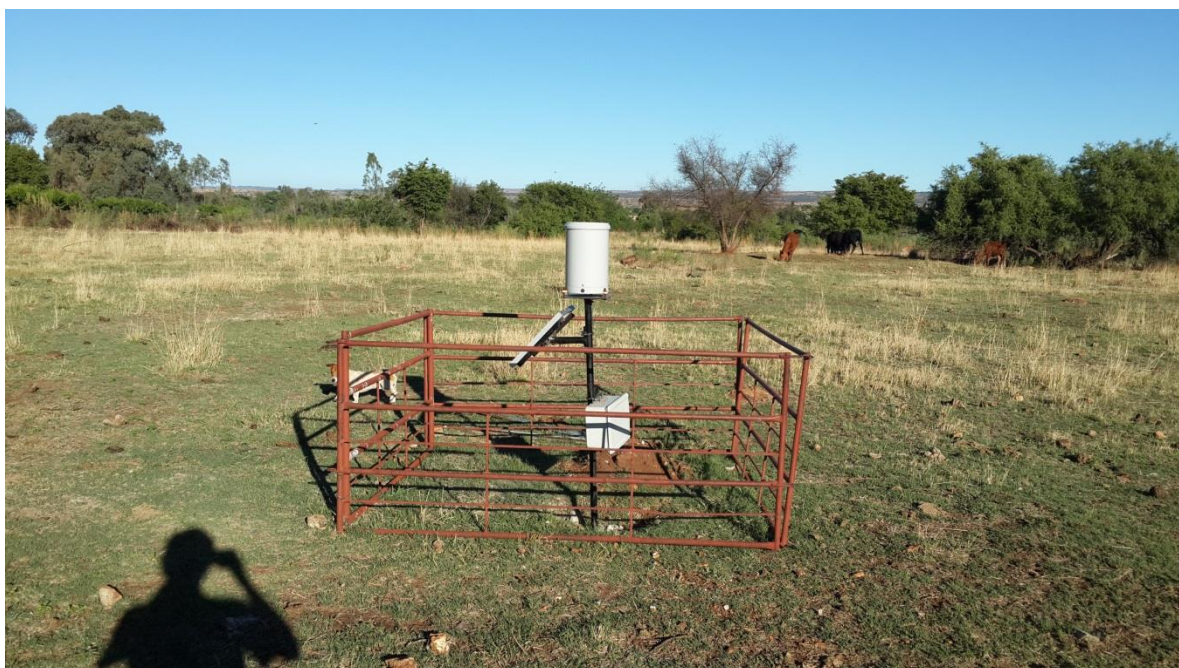
Figure 2-12: The Muiskraal gauge is fenced off to deter livestock from disturbing it.
