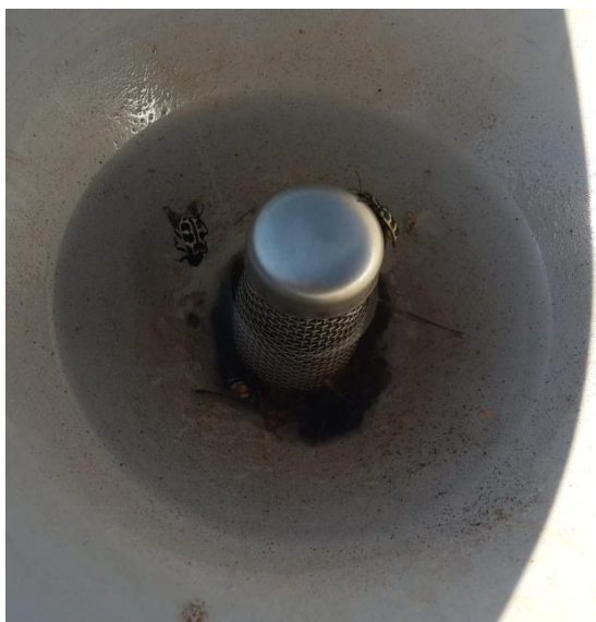
Figure 2-14: The Leriana gauge, totally blocked due to a spider's nest inside the syphon.
