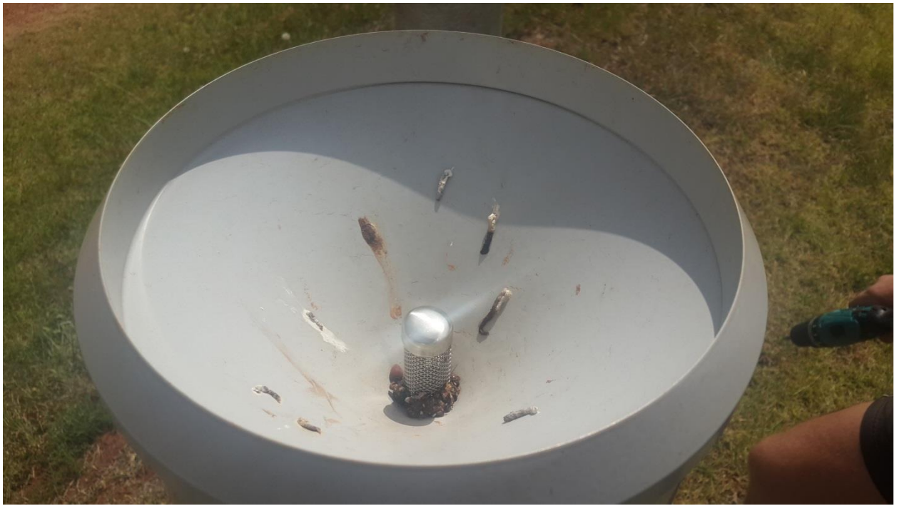
Figure 2-8: The catch filters of the TB 3 keeps debris and insects out of the mechanisms of the gauge.
