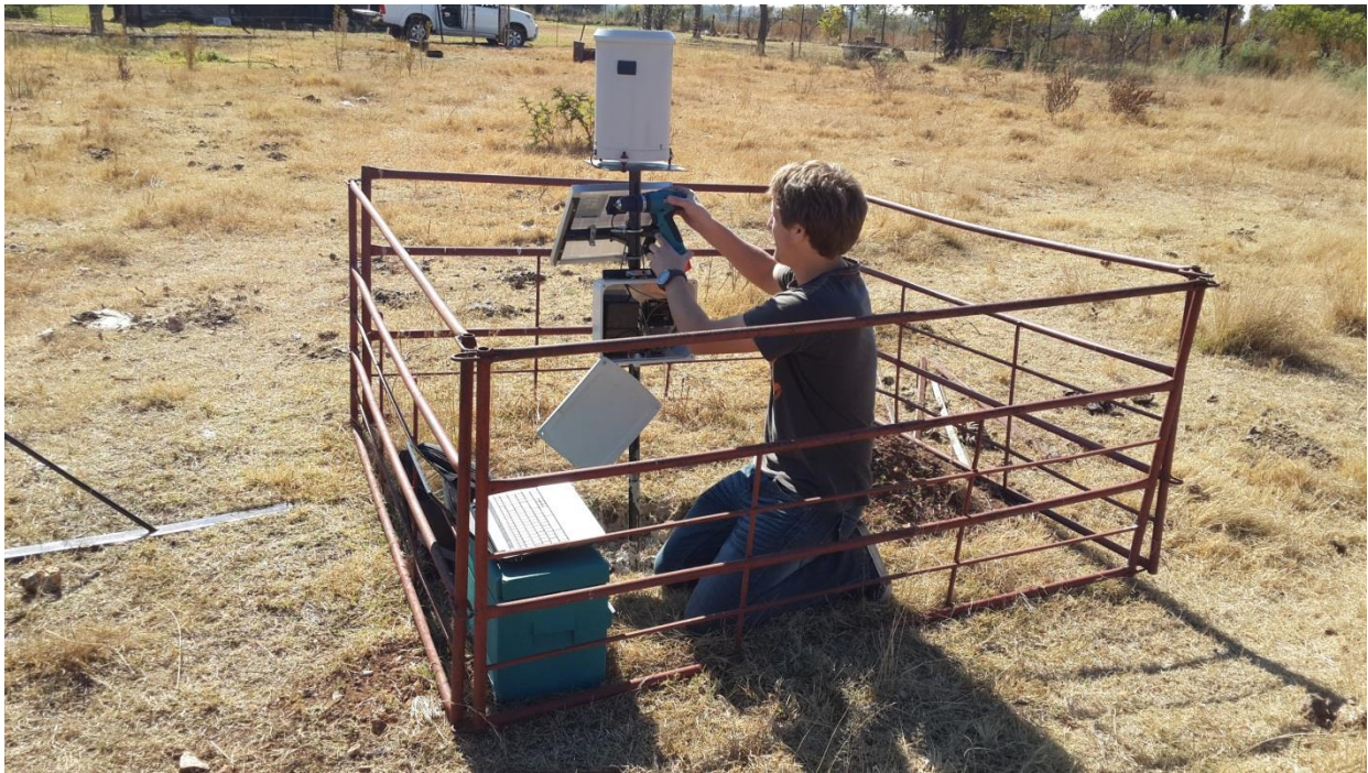
Figure 2-15: Retrieving data and setting the time and date on the data loggers of the MRGN.
