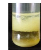
Figure 4: Emulsification of kerosene by B. cereus in the presence of heavy metals
