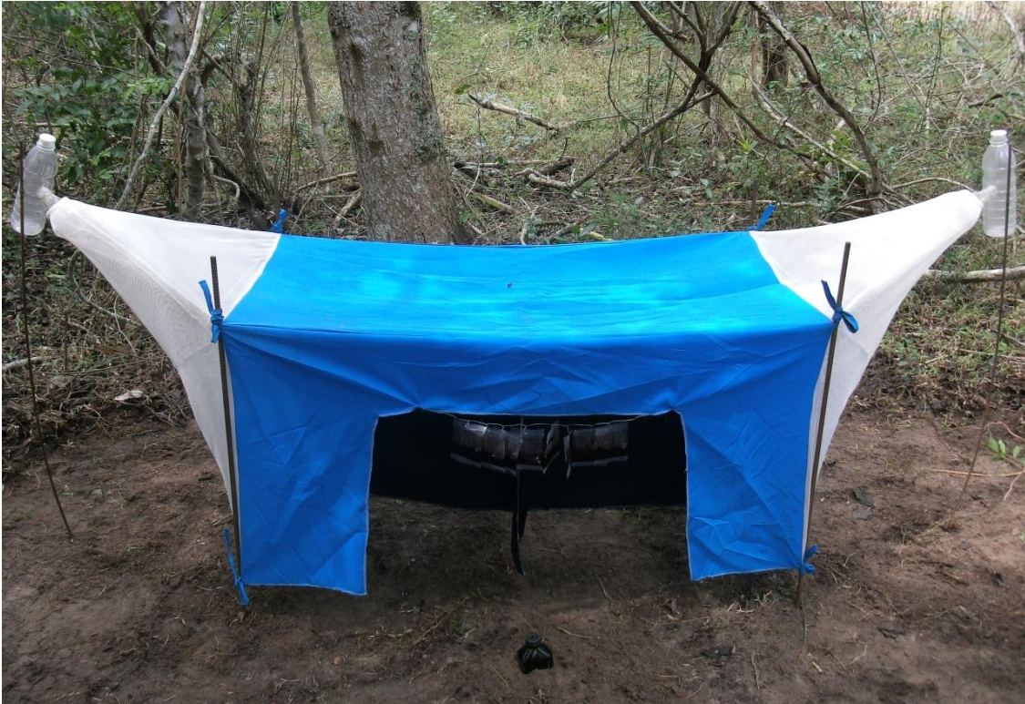
Figure 6a: H-trap used to capture tabanid flies in Lesotho and in South Africa.
