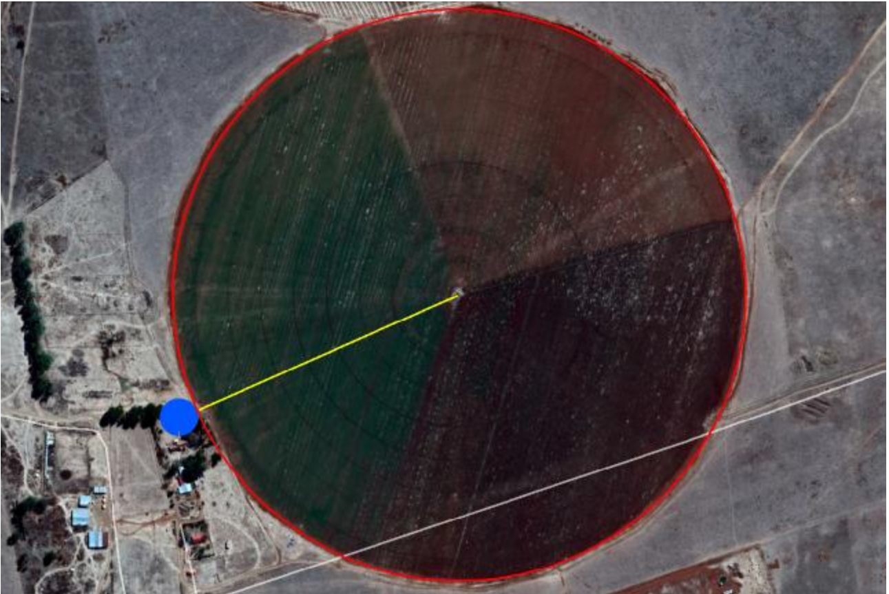
Figure 3.1 Aerial View of the Irrigation System, showing the Dam (Blue), Pipeline (Yellow) and Centre Pivot (Red).
