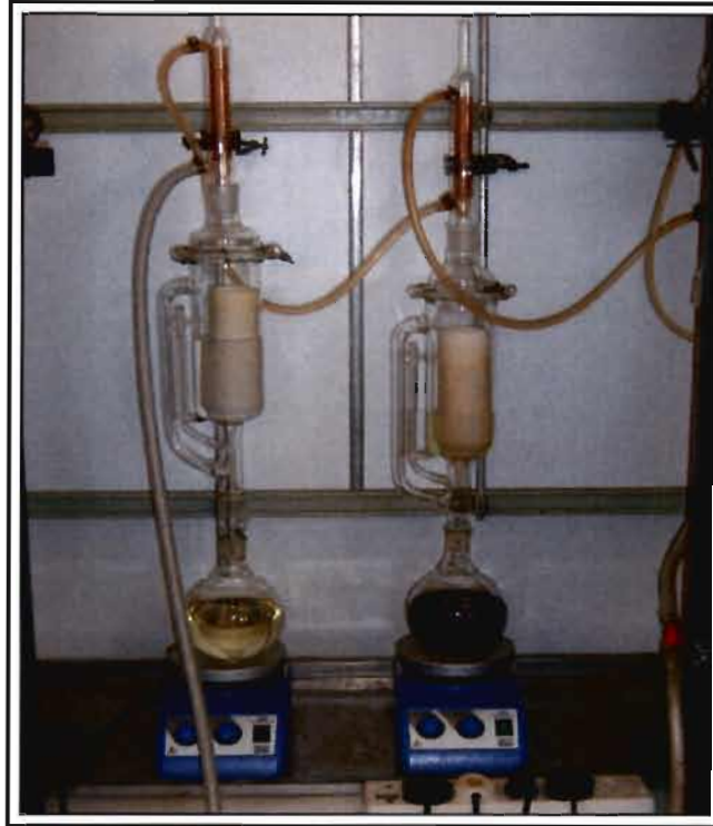
Figure 3.5 The Soxhlet apparatus set-up in laboratory.
